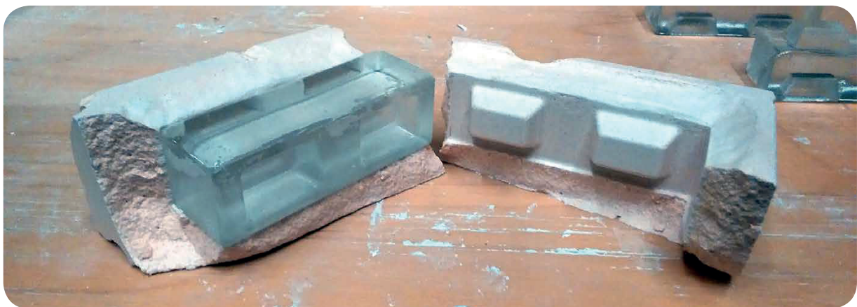
Figure 55: Disposable Silica Plaster Mould, source: (Oikonomopoulou, 2019)
