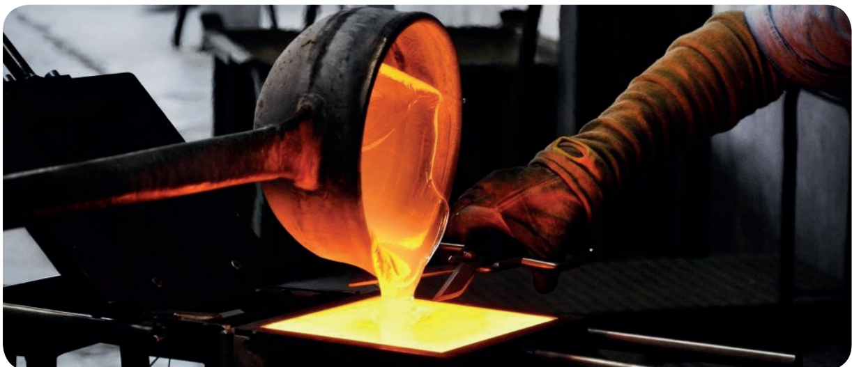
Figure 32: The molten glass is manually casted in the mould, source: (Oikonomopoulou, 2019)
