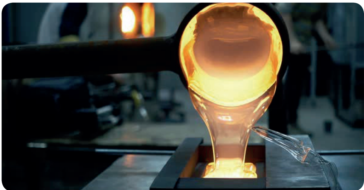
Figure 33: Primary casting process of hot forming or melt quenching, source: (Dissolve, n.d.)
