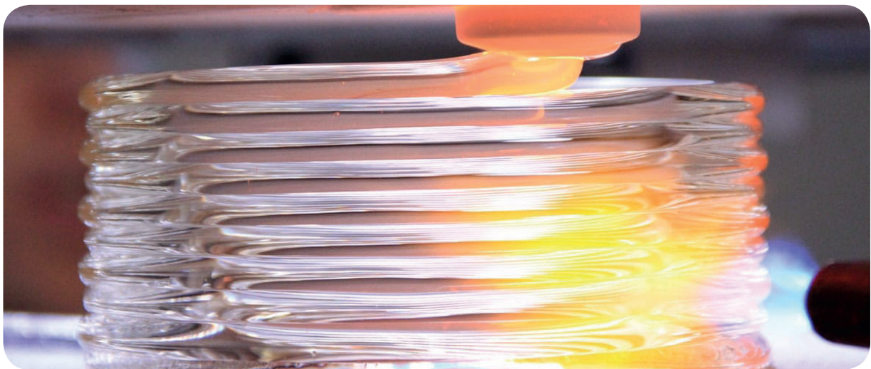
Figure 30: How the layers of glass are placed on top of each other, source: (Llowlab, 2015)
