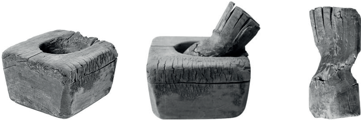
Figure 76: An original, damaged, empolion of the Parthenon. The damage is probably caused by an earthquake, source: (Karakitsou & Konteas, 2013)
