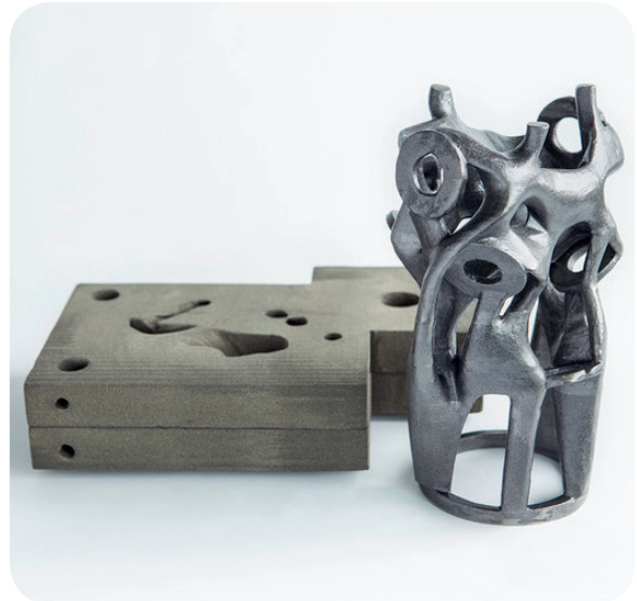
Figure 57: 3d printed sand mould to cast a steel node, source: Davidfotografie from (Niehe, 2017)
