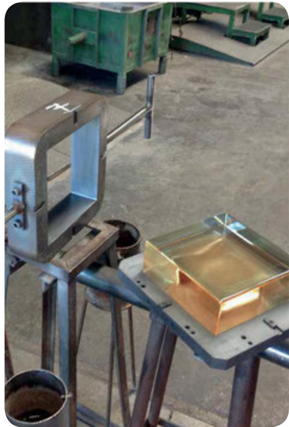
Figure 54: High precision, permanent steel moulds for the Crystal Houses project, (Oikonomopoulou, 2019)
