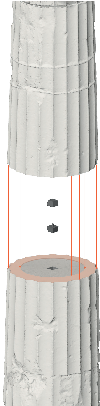
Figure 112: Structural principle of the original connection between two marble drums where all load is transferred at the periphery
