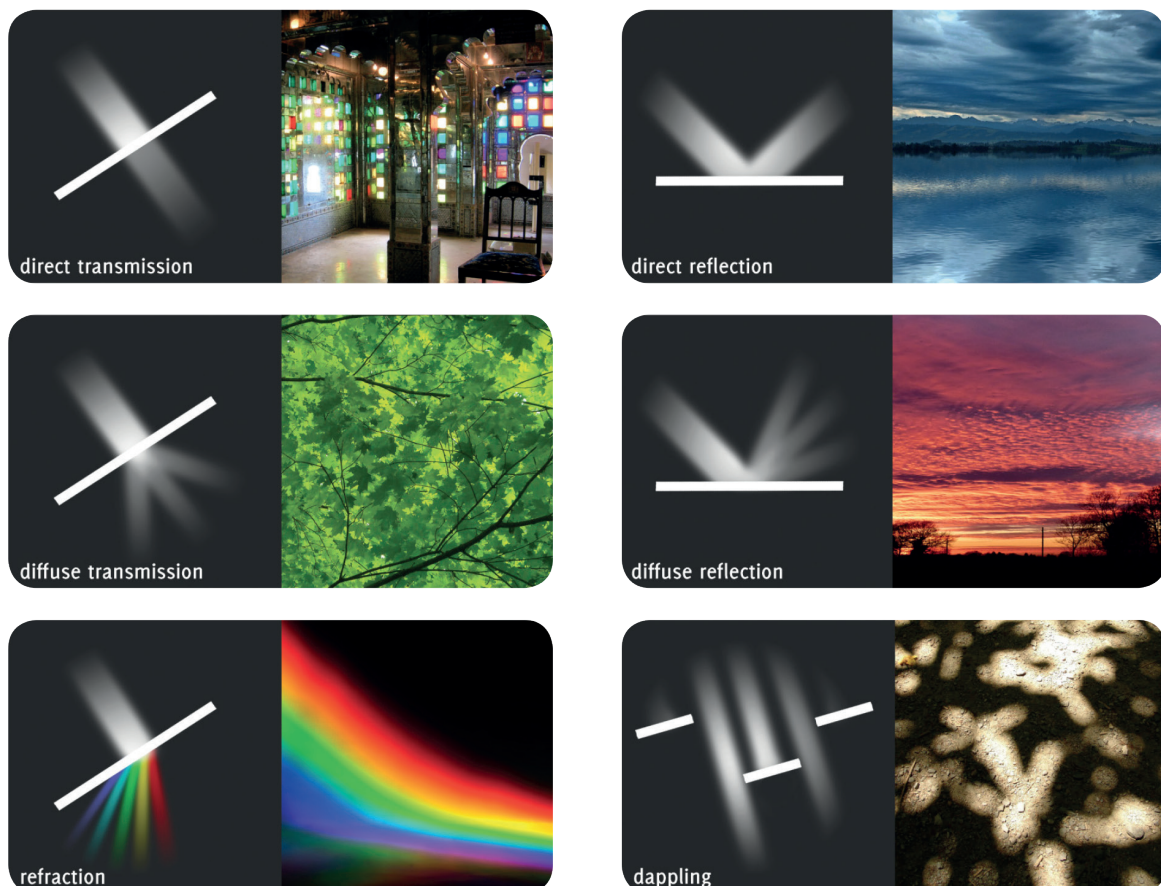
Figure 82: Most common optical phenomena, source: (Barou, 2016)
