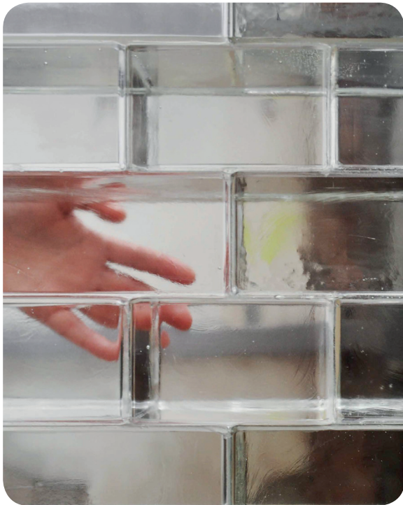
Figure 84: The transparency of the Crystal Houses facade cannot be reached with the given geometry of the column, source: (Oikonomopoulou, 2019)
