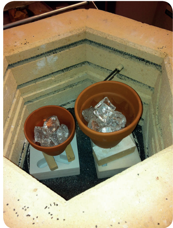
Figure 34: The secondary process of kiln casting, source: (Oikonomopoulou, 2019)
