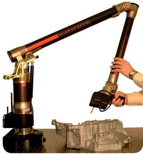
Figure 42: Example of a manual contact scanner, source: (Langnau, 2015)
