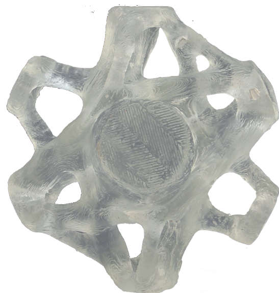
Figure 88: Structurally optimised glass node, source: (Damen, 2019).
