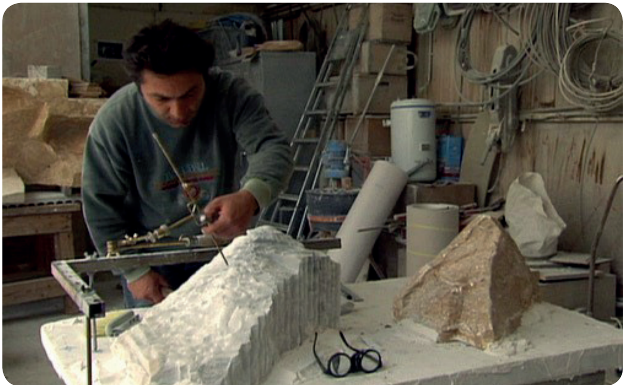
Figure 79: A master stonemaker is manually carving a new piece of Pentelic marble, using a pantograph and a cast plaster replica, source: (Glassman, 2008)
