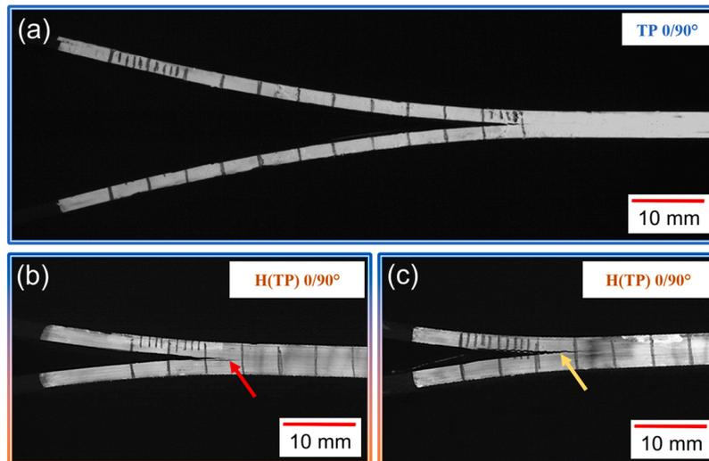
**Fig. 3.** Exemplary images of crack propagation during DCB tests for H(TP) 0°/90° hybrid laminates (b and c) in comparison to the corresponding sample TP 0°/90° (a). Forming of parallel cracks (b, red arrow) and crack jumping (c, yellow arrow) indicate a pronounced change in crack propagation mechanism at an early state of crack growth in comparison to the pure TP sample.
