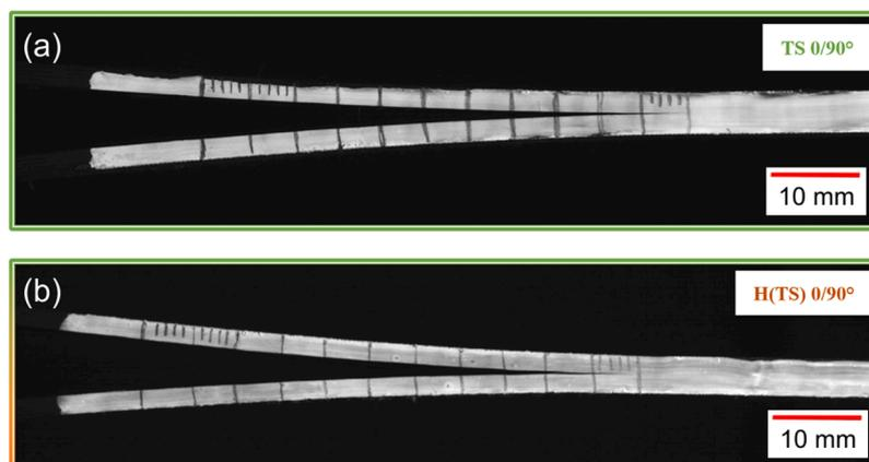
**Fig. 2.** Exemplary images of crack propagation during DCB tests for H(TS) 0/90° hybrid laminates (a) in comparison to TS 0/90° (b). There is no evidence for a change in crack propagation mechanism confirming the  $G_{Ic}$  values on a comparable level.
