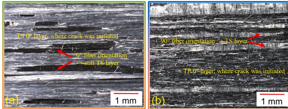
**Fig. 7.** Fractography of tested laminate configurations: view on the upper half of the cracked sample. In H(TS) 0/90° the crack does not reach the adjacent TP layer (a), which is clearly the case for H(TP) 0/90° (b).
