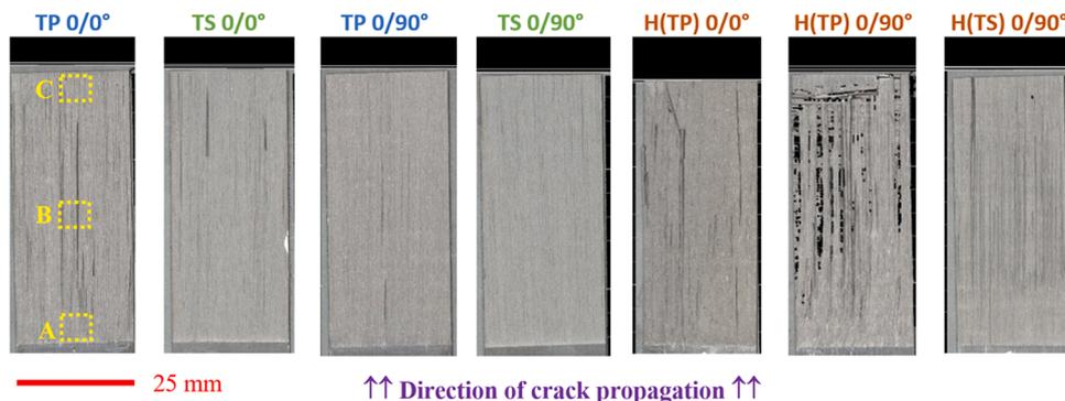
Fig. 6. Fractography of tested laminate configurations: view on the upper half of the cracked sample. Width of every sample displayed is 25 mm. Black spots in H(TP) 0/90° indicate the visibility of the 90° TS layer. The yellow squares mark the positions of the roughness measurements (see below).
