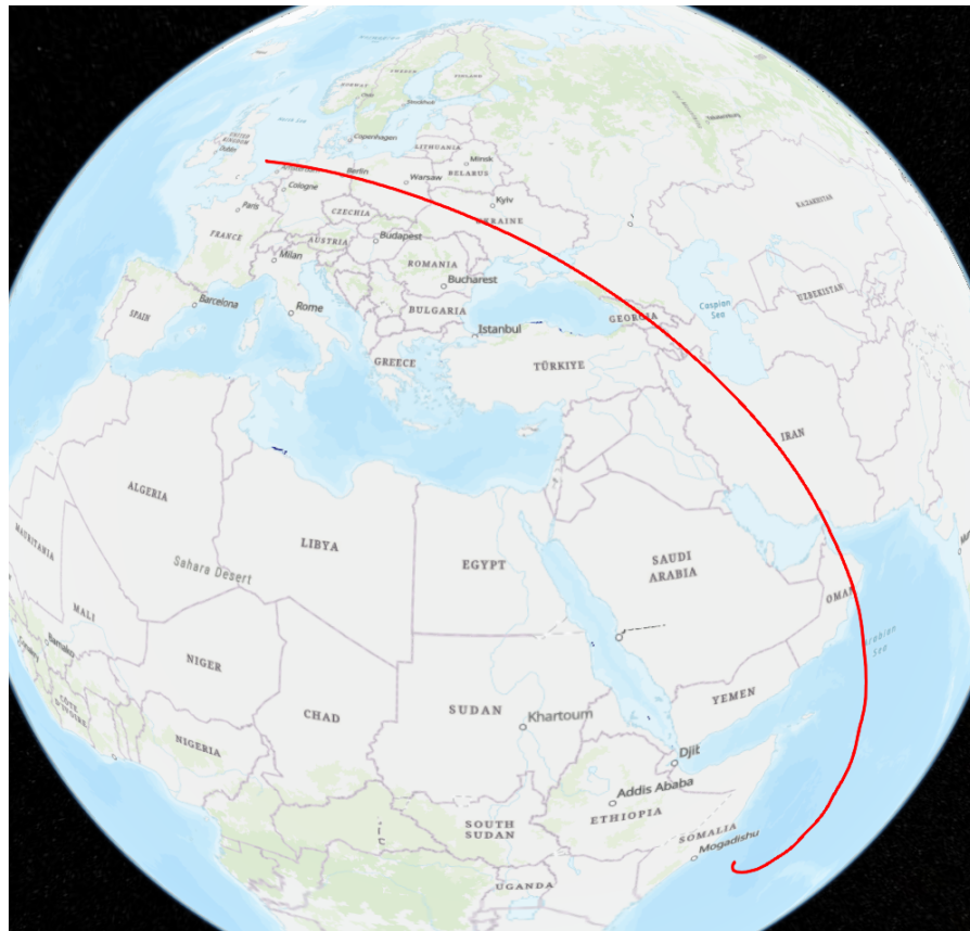
Figure 5.7: Trajectory of HGV with bank angle 30^\circ .
