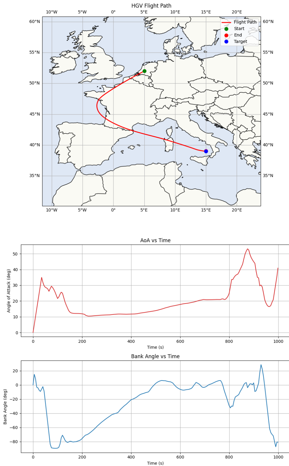
Figure 6.34: Ground trajectory and control variable inputs to navigate towards arbitrary target point.
