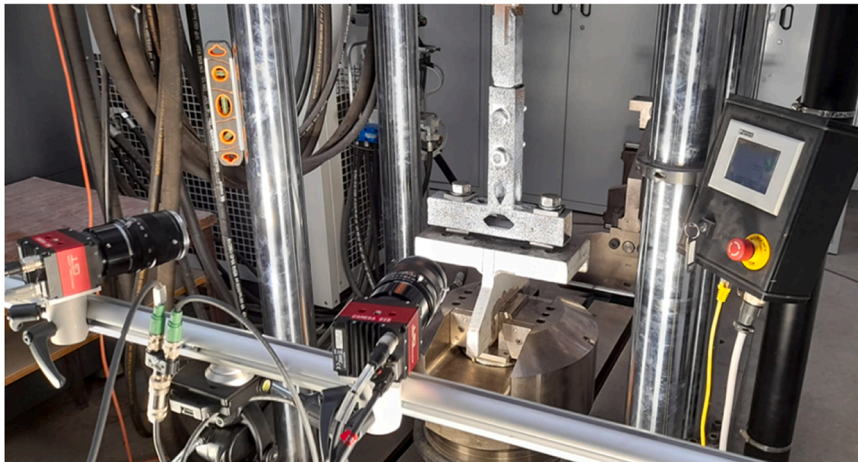
Fig. 33. Experimental test of the optimized T-joint CB1.
