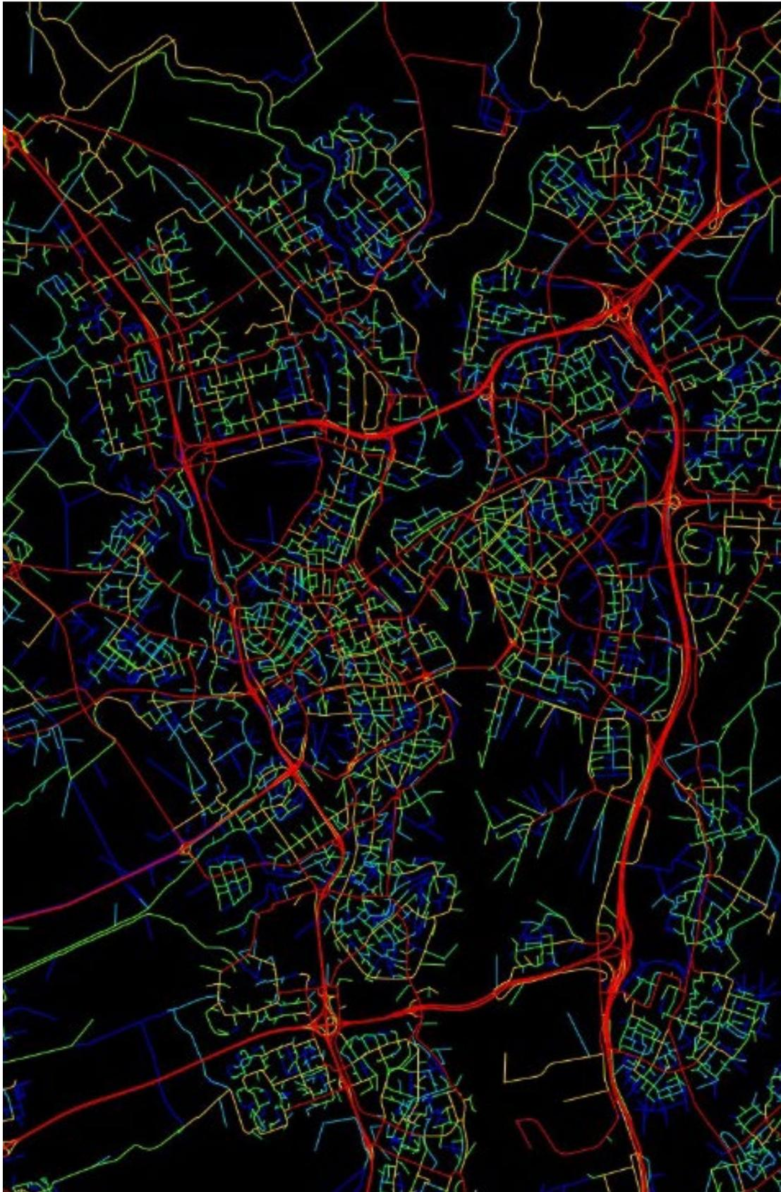
Figure 41, Predicted average hourly traffic load map of Rotterdam
