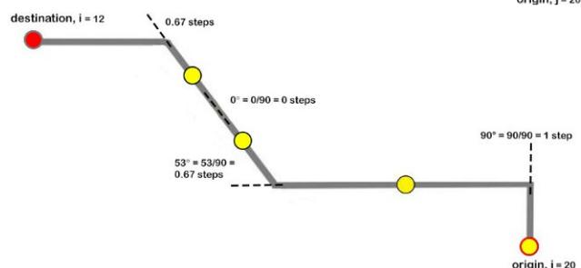
Figure 8, Least Angle Change Path: angular distance (weighted topological distance),  $d_{ji} = 196^\circ = 196/90 = 2.18$  topological steps
