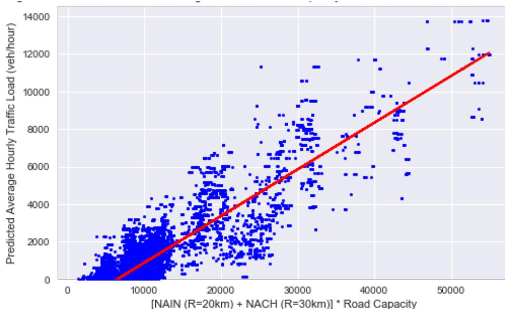
Figure 42, scatterplot with the sum of weighted NAIN (radius = 20 km) and NACH (radius = 20 km) by road capacity
