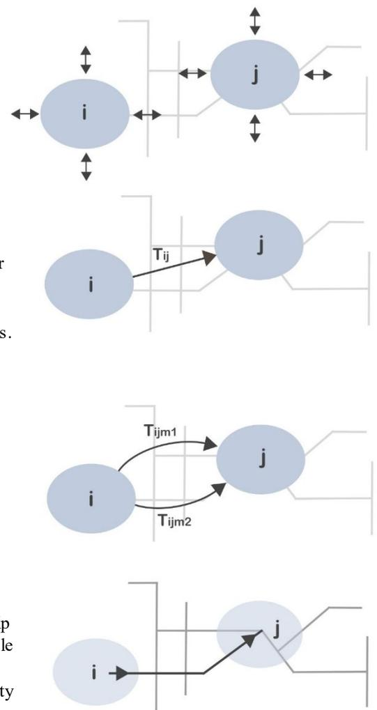
Figures 17, 18, 19 and 20 (From top to bottom), Principle diagrams of Four Step Macroscopic Traffic Model
