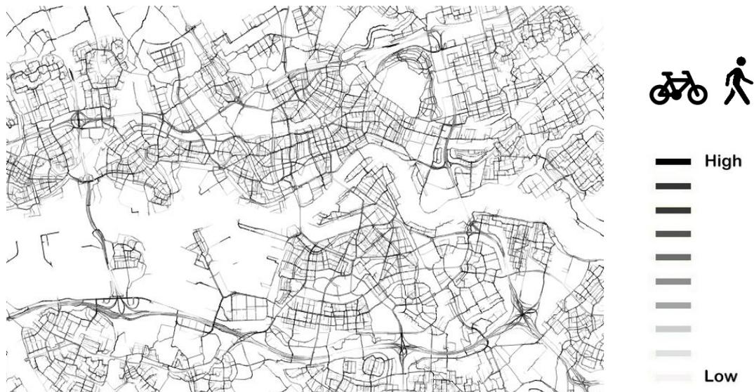
Figure 9, Local (Angular) Betweenness Centrality of Rotterdam (radius = 1000 m)
