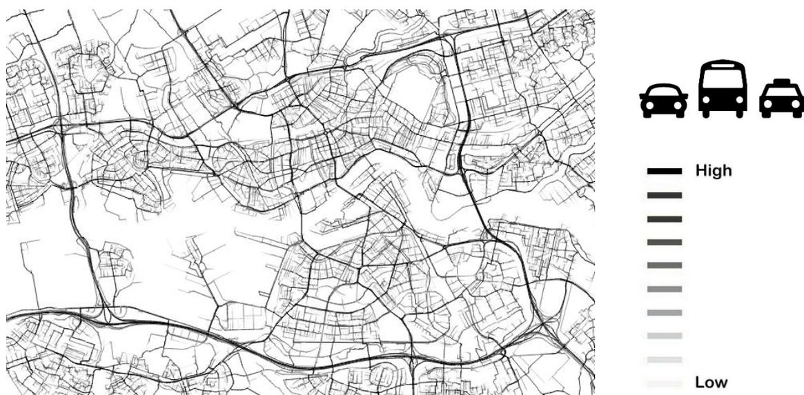
Figure 10, Global (Angular) Betweenness Centrality of Rotterdam (radius = 30 km)
