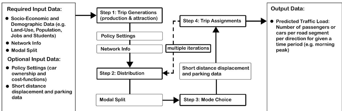
Figure 22, Four Step Macroscopic Traffic Model Data and Approach
