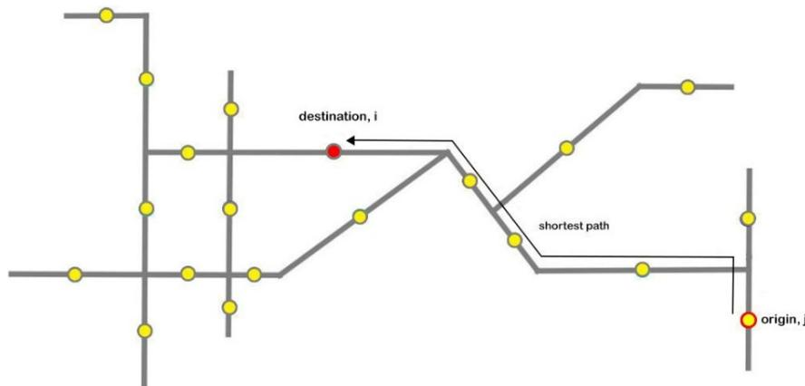
Figure 5, The shortest path from origin node (j) to destination node (i)
