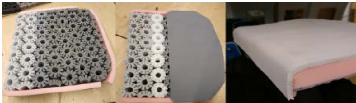
Figure 8 seat prototype. Spring-foam distribution (left), firm layer addition (centre), final cushion without upholstery
