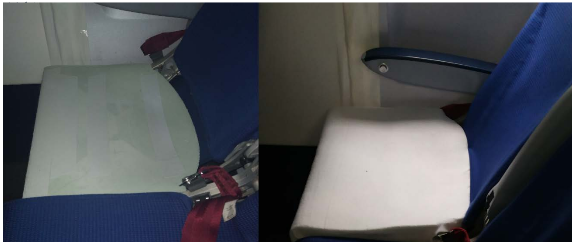
Figure 9: Hard-foam CNC made bottom plate attached to seat frame (left,) prototype, cushion attached to bottom plate (right)
