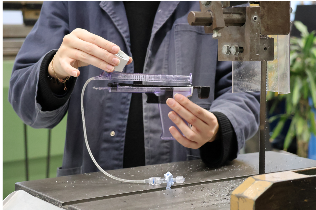
Figure 49. Everest inflator after being sawed in two halves.
