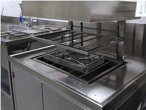
Figure 30. Mechanically cleaning with an ultrasonic cleaner.
