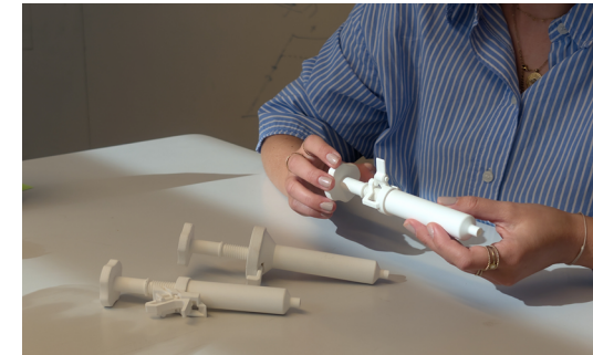
Figure 84. Concept 1 (overcentre) being evaluated with a student on ease of dis- and reassembly, and ease of use.
