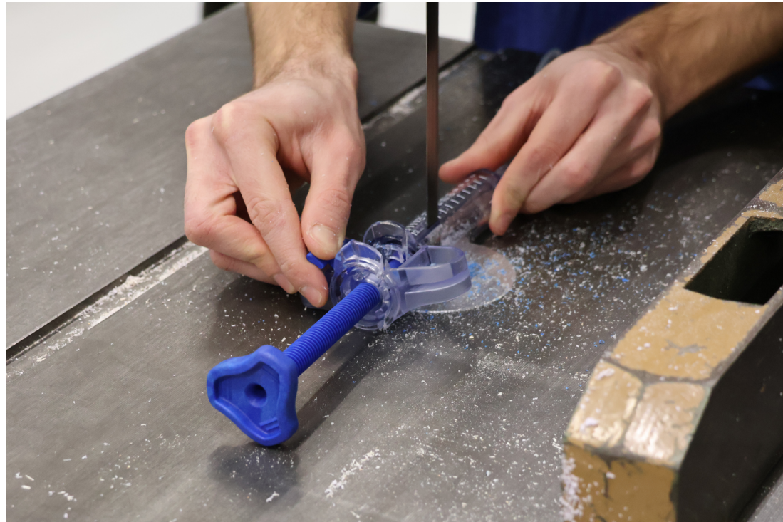
Figure 41. Final disassembly destructive method used for the Encore™ 40: a saw machine. As can be observed, this destructive method produces quite a lot of debris, which probably slightly influences the weighting of the parts for economic and environmental assessment.
