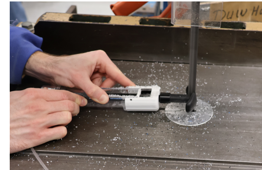
Figure 51. Vedkang™ going through a second sawing cycle after separating the actuator.
