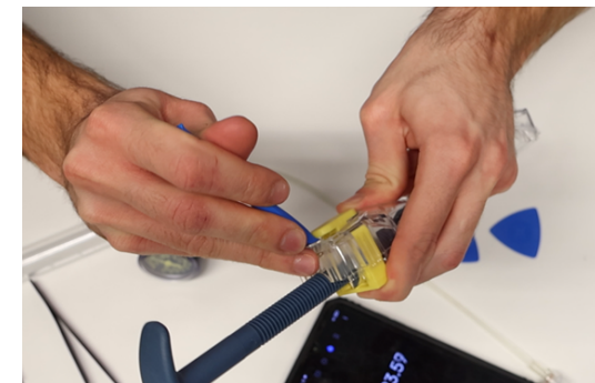
Figure 38. Separating the actuator (8) from the half-nut (10) of the Encore™ 26. The gap to introduce the spudger was so small that I ended up hurting myself.
