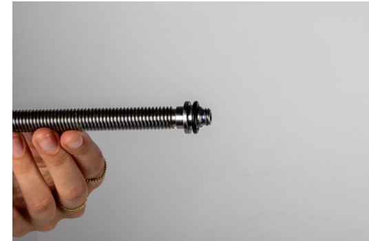
Figure 94. 3. Place the O-ring to in the plunger. Expand it uniformly.
