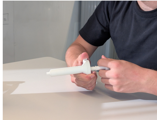
Figure 86. Concept 3 (springs) being evaluated with a student on ease of dis- and reassembly, and ease of use.
