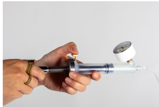
Figure 99. 8. Thread the connector into the barrel and it is ready to operate.
