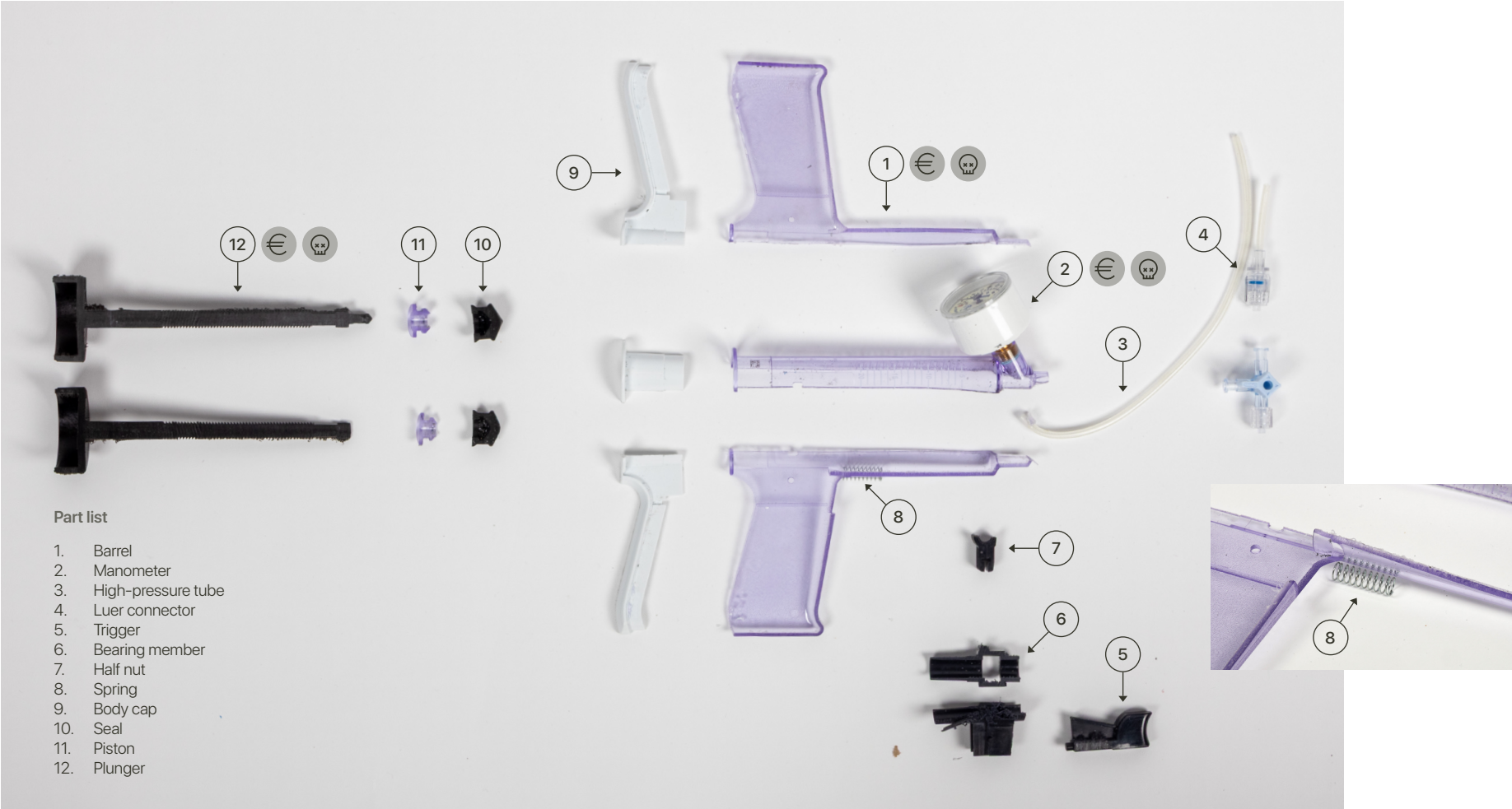
Figure 50. Disassembled Everest inflator. A part list is included. The parts are numbered and the environmental and economic hotspots are highlighted.
