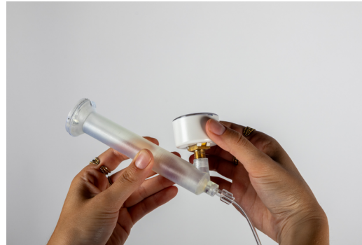
Figure 93. 2. Insert the O-ring and thread in the manometer for a liquid-tight connection.
