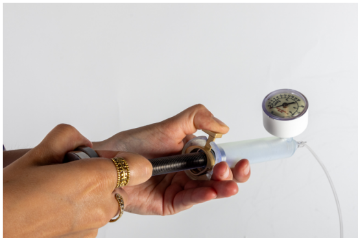
Figure 98. 7. While pressing the half nut, push the plunger inside the barrel.
