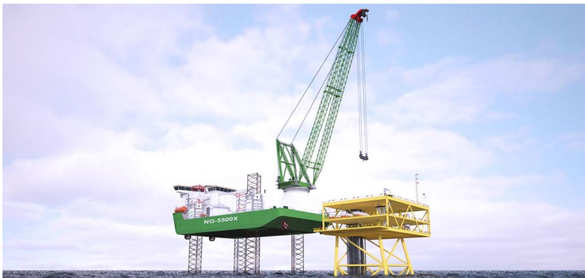
Figure 3.12: Jack up barges are now often used for wind park installations, but could play a role in jacket decommissioning in shallower waters. (Picture from *gustomsc.com*)
