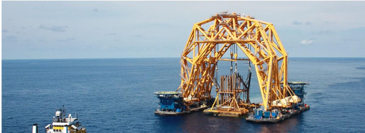
Figure 3.11: The Versabar heavy lifter now active in the Gulf of Mexico is a non conventional heavy lift method which could be used for jacket removals. (Picture from *versamarine.com*)
