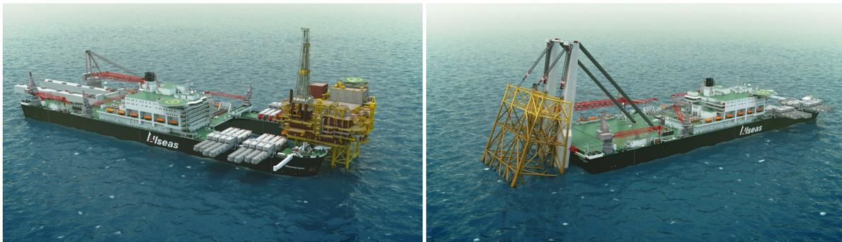
Figure 1.3: The Pioneering Spirit is the only known application of the single lift decommissioning method for very large platforms (picture from allseas.com).
