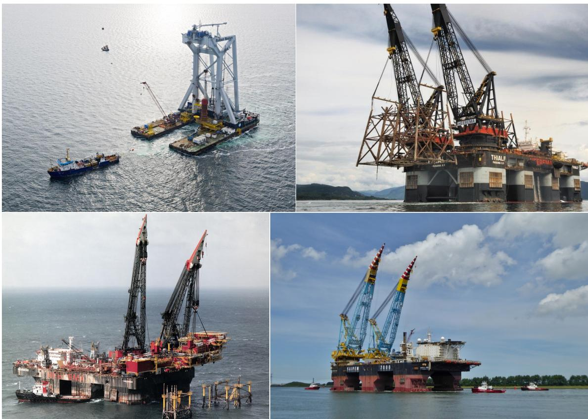
Figure 2.9: The single lift competition in the North Sea for the buoyancy concept up to 7,500 MT (f.l.t.r.: Svanen, Thialf, Hermod and Saipem 7000, pictures from *images.google.com*)
