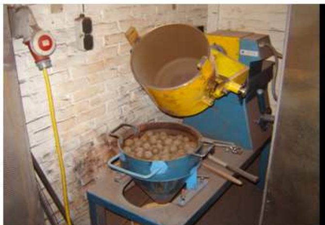
Figure 5.9 Bond ball mill used in feed preparation
