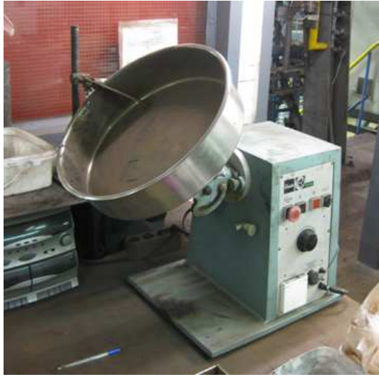
Figure 5.11 Lab scale balling disc used during balling
