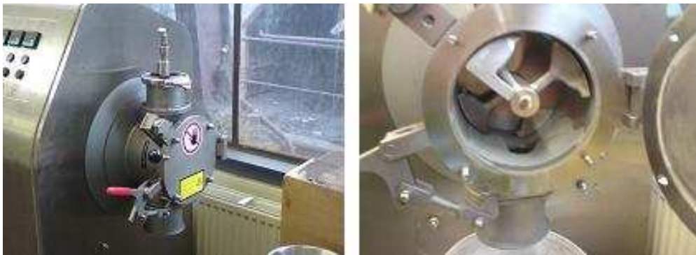
Figure 5.12 Lab Sclae Lödige™ mixer used during experiments outside (left) inside (right).
