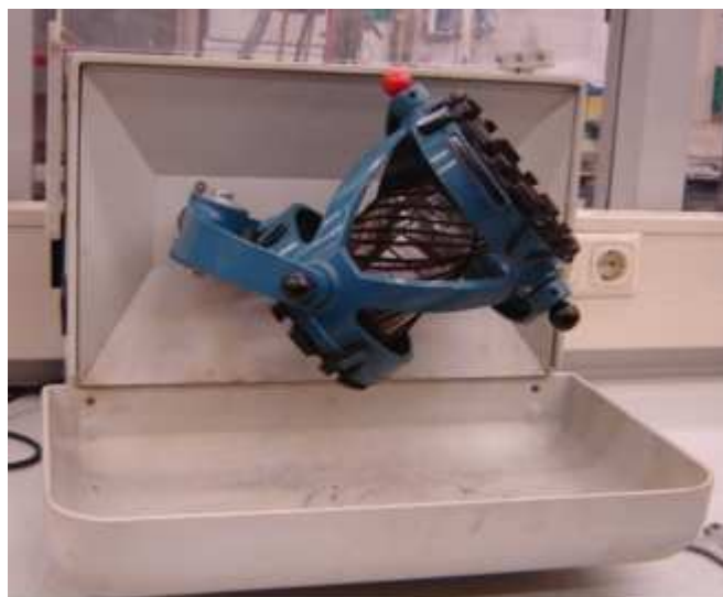
Figure 5.10 Turbula© powder mixer used during feed preparation.
