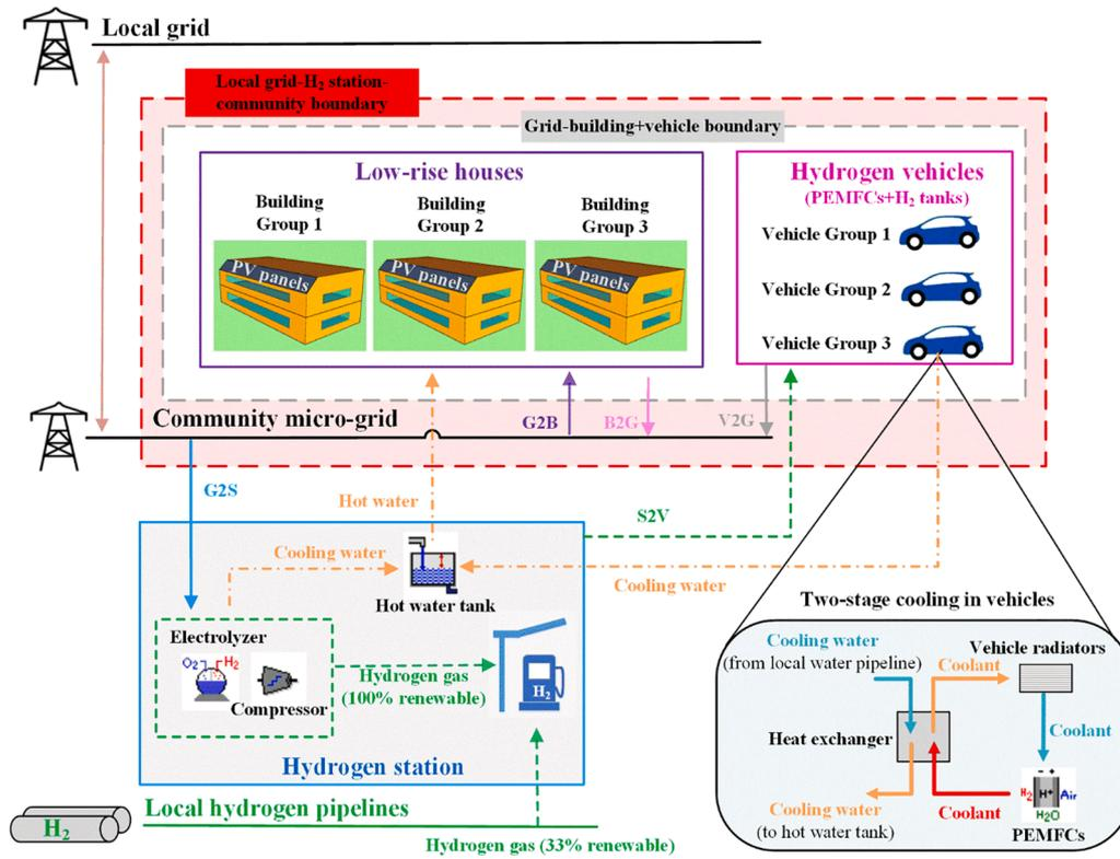
Fig. 5. The structural configuration of a community integrating low-rise residential buildings, rooftop PV systems, fuel-cell-powered HVs, an adjacent H<sub>2</sub> station, local hydrogen pipelines, community micro-grid, and local power grid. (G2B means the grid-to-building interaction; B2G means the building-to-grid interaction; G2S means the grid-to-H<sub>2</sub>-station interaction; S2V means the H<sub>2</sub>-station-to-vehicle interaction; V2G means the vehicle-to-grid interaction.)
