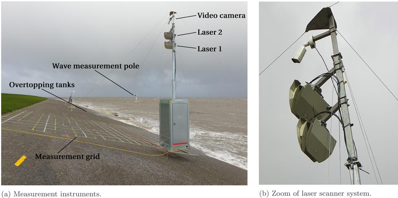
Figure 2: Left: New laser scanner system on the dike in the Eems-Dollard estuary, next to the overtopping tanks, during storm Ciara. The Rijkswaterstaat (wave) measurement pole can be seen in the distance. Rijkswaterstaat is the Directorate-General for Public Works and Water Management in the Netherlands. Right: From the bottom to the top, Laser scanner 1, laser scanner 2, video camera.
