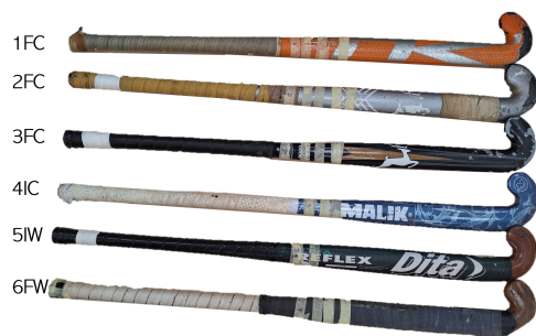
Figure 3.1: Measured sticks - a set of used field (F) and indoor (I) hockey sticks made of carbon (C) or wood (W)
