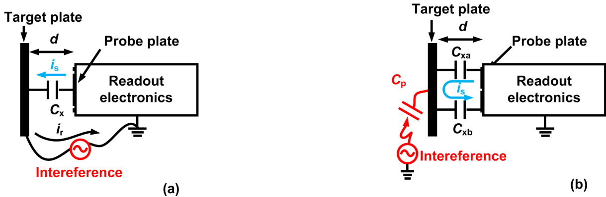
Figure 1.1 (a) Conventional capacitive position sensing system, in which the closed loop incorporates the target electrode and the input of the interface electronics; (b) Push-pull capacitive position sensing system with floating target electrode and significantly reduced closed loop incorporating only the sensing electrodes.
