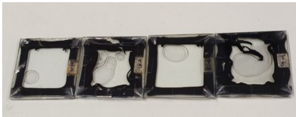
Figure 3.1: Damp heat tests of several fluids (left to right: PDMS, Electrocool, Mivolt, Opticool) between two glass sheets sealed with PIB sealant. Electrocool and Opticool show bad material compatibility with PIB, as PIB dissolves in the fluids, tested by Urvashi Bothra at TU Delft.
