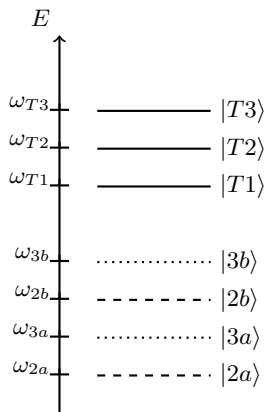
FIG. 2. Schematic representation of the energy spectrum of the Hamiltonian in Eq. (2). This spectrum only contains the ‘single-photon levels’, i.e., the levels that are accessible only by absorbing one single photon (plus |T2\rangle , for completeness). Energy levels represented with solid lines are coupled only to the incoming transmission line. Dashed lines describe levels coupled to the second outgoing transmission line and also the incoming one. Dotted lines describe levels coupled to the third outgoing transmission line and also the incoming one. The separation of the energy levels is not to scale.
