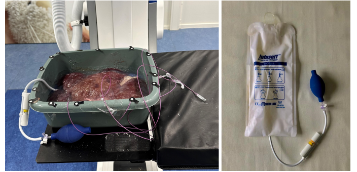
Figure 5: The setup for the respiratory motion simulation experiment. The medical infusion pump sachet shown on the right is positioned underneath the liver.
