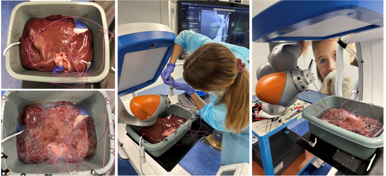
Figure 2: Preparing the setup. F.l.t.r.: The top left picture shows the liver positioned on the latex gloves, in pink the endovascular catheters - the bottom picture shows the liver fixated with agar - the middle picture shows preparing the liver by inserting agar spheres - the right picture shows the robot arm before needle insertion. The black and white stickers on the liver are the markers for ClarifEye.
