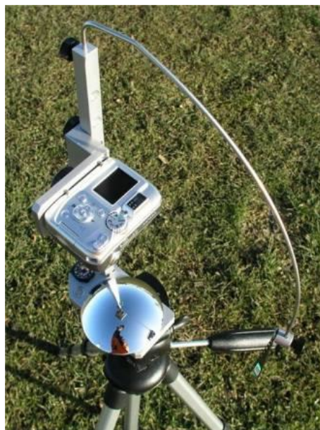
Figure 2.6: HORIcatcher tool to calculate the skyline profile, from [24].
