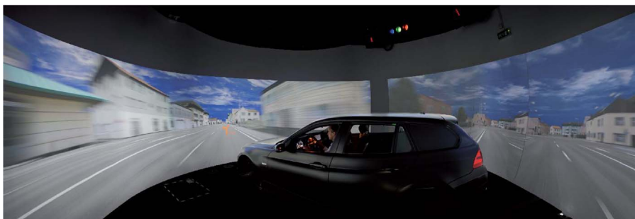
Fig. 5. Dome of the high-end moving base driving simulator (Source: BMW AG).
