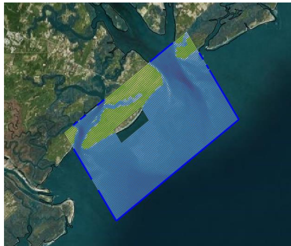
Figure 13: Location, lay-out and size of the computational grid that is used in used in both the FLOW and WAVE module. The grid cut-out represents the size and location of the finer nested grid.
