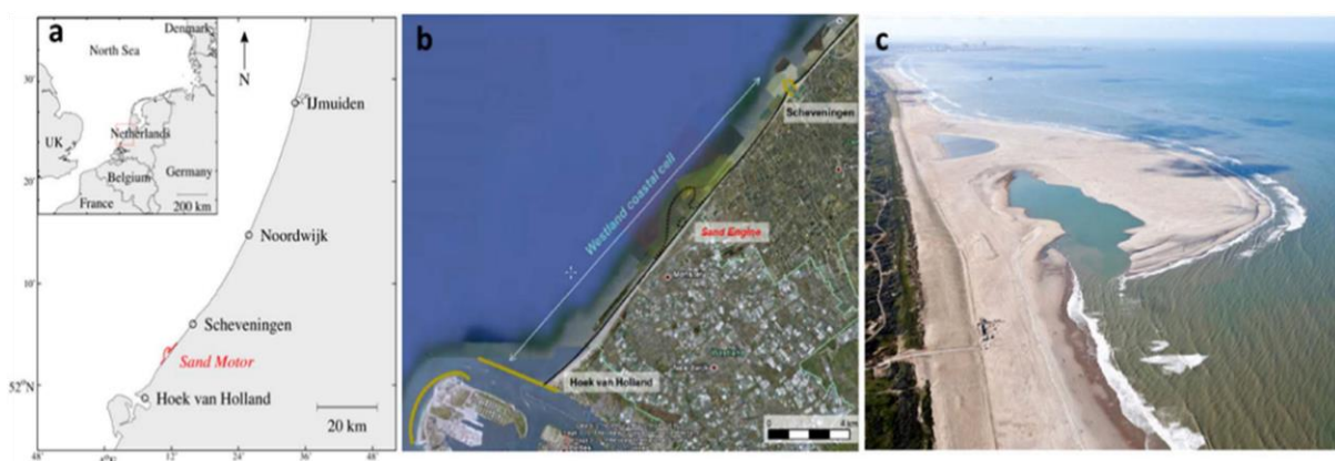
Figure 10: A: Location of the Sand Engine (Sand Motor) at the Dutch coast. B: The Delfland coastal cell including a sketch of the Sand Engine. C: The Sand Engine after completion in 2011. (Source: Luijendijk et al., 2016)
