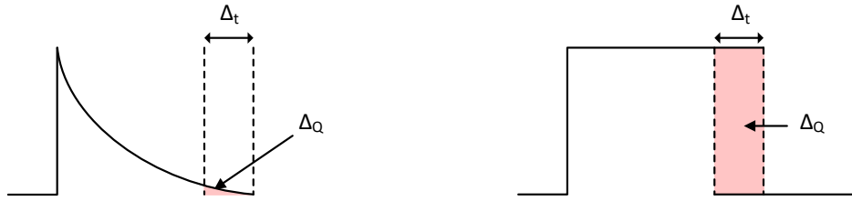
Figure 4-6: Effect of jitter on SC DACs (left) and CT-DACs (right).
