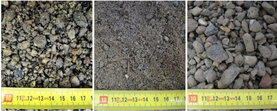
Figure 4.35: Concrete granulate input, fine and coarse product
