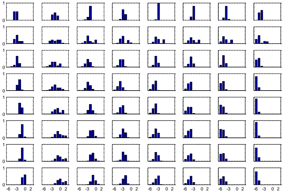
Figure A.7: Distribution of the order of collision probability of each size fraction pair
