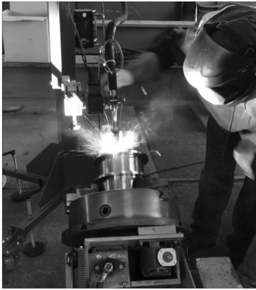
Fig. 3. Specimen welding using a robot with a turning manipulator and a fixed torch.
