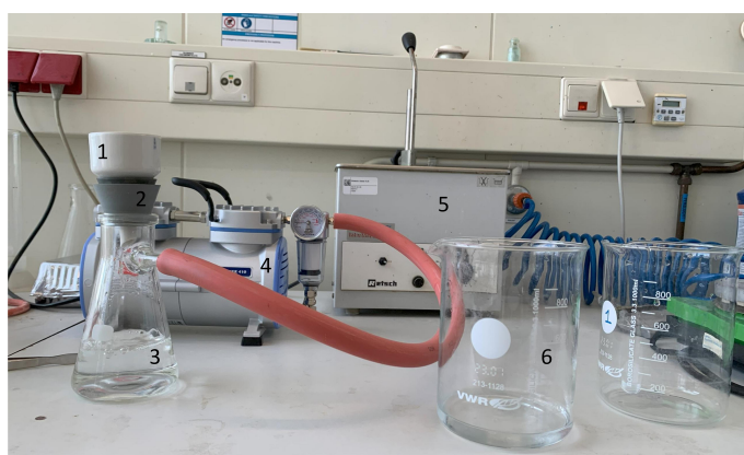
Figure 3.11: Gravimetric method filter setup
