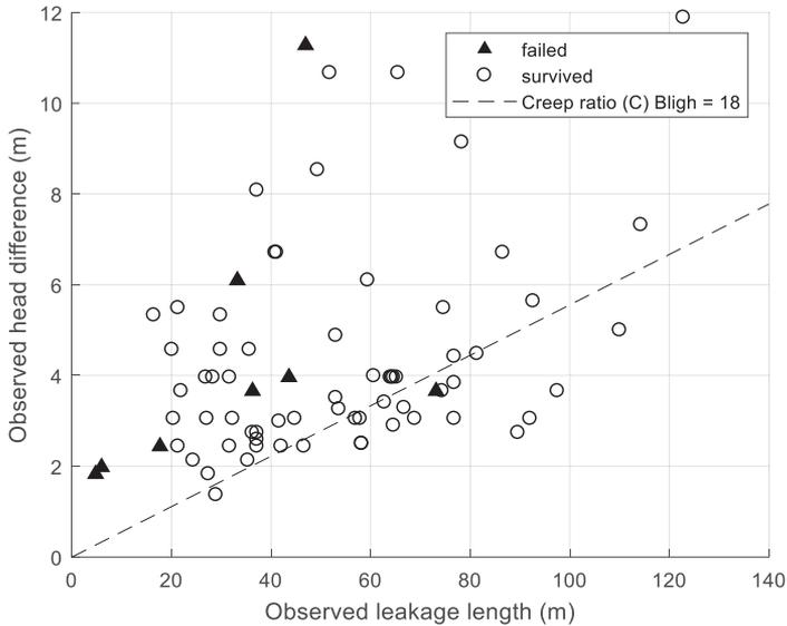
**Figure 1.** The data of Bligh for sand, fine sand and silt, failed and survived, plotted against the proposed Creep ratio C= 18.
