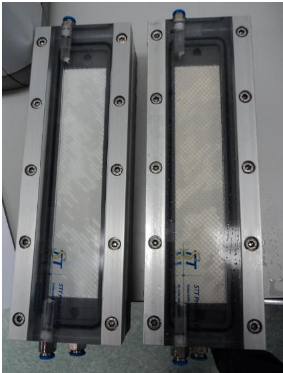
Figure C-1 - Visual observation of MFS placed after GAC experiment 6 (without RO) (left) and MFS placed after post-filter 6 (with RO) (right)
