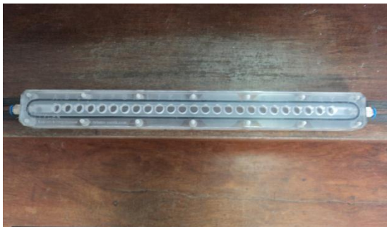
Figure 3-4 - Modified Robbins Device to simulate biofilm formation
