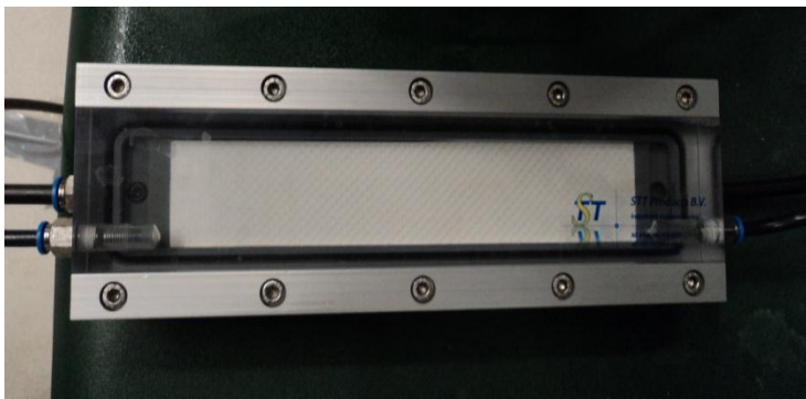
Figure 3-2 - Membrane Fouling Simulator for investigating (bio)fouling potential of water
