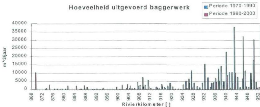
Figure 16, locations of dredged volumes per year for the Bovenrijn and Waal. Two periods are shown; 1970-1990 (blue) and 1990-2000 (red) (source: RIZA, 2001)
