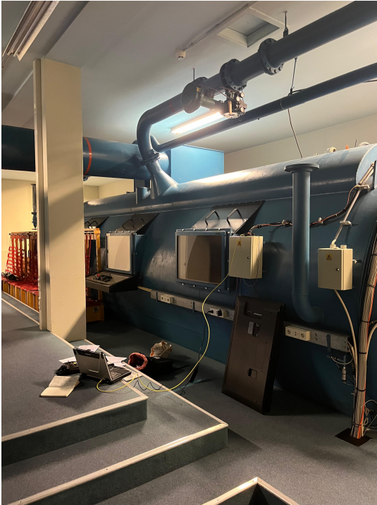
Figure 3.1: The CML hypobaric chamber. The glass window through which the test box is visible is shown.
