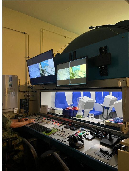
Figure 3.2: Control panel used to regulate chamber pressure via equivalent flight altitude.
