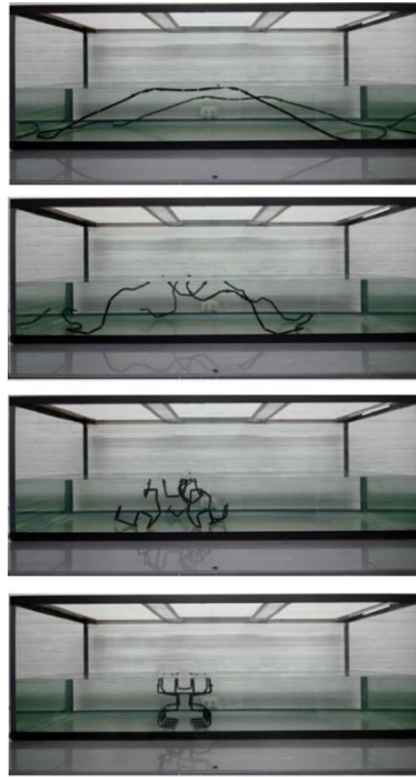
Figure 149: A complex structure emerges from the 4D printed rods when submerged. 43
