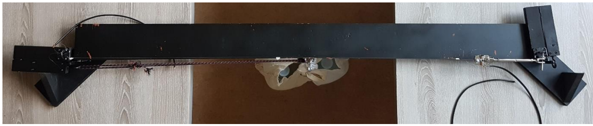
Figure 118: The new set-up, which uses one SMA per rotating arm. The left is active in this photo, whilst the right arm is not
