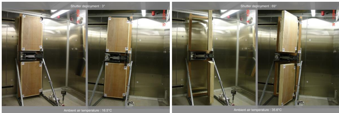
Figure 37: adaptronic temperature-sensitive panels that use paraffin-based thermal passive actuators. A stroke angle of 66 degrees is achieved using a temperature difference from 16.5°C to 35.6°C
