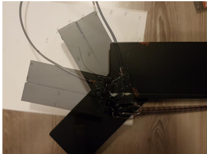
Figure 122: Testing the actuator stroke performance for the 6kg, 4-8mm prestrain, which resulted in a 49.8° angle
