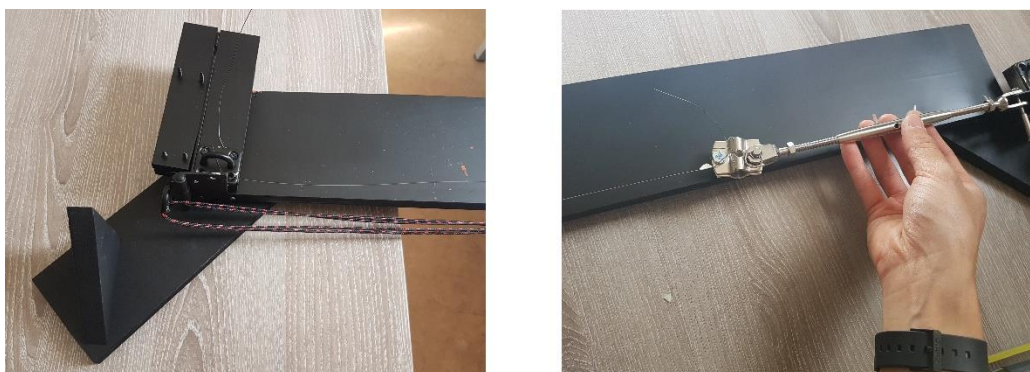
Figure 120: The attachment to the left and right SMA ends. The right hand side is now fixed to a stationary point instead of to the other rotating arm, with a turnbuckle to allow adjustment.
