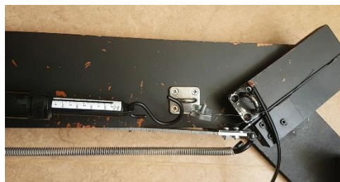
Figure 125: testing the force transmission loss between spring and SMA, due to the hinge
