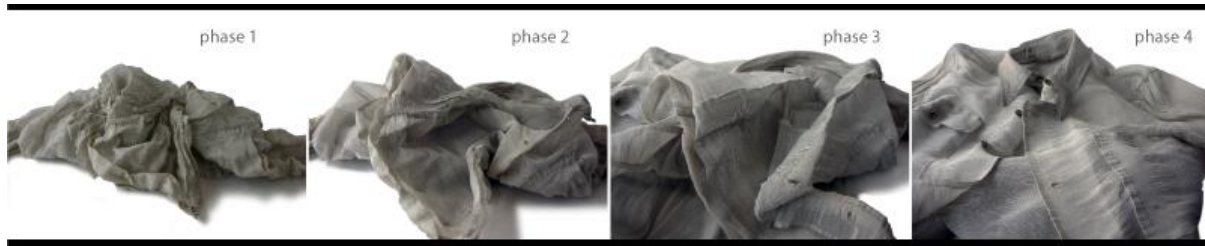
Figure 21: A shirt developed by Grado Zero Espace that self-rolls its own sleeves up in hot temperatures, made of Shape Memory Alloy (Grado Zero Espace).
