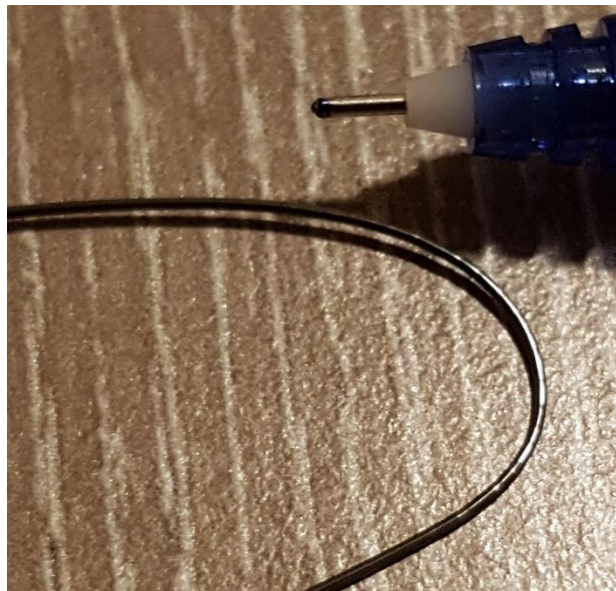
Figure 110: Very subtle differences in colour along the length of this partially transitioned SMA
