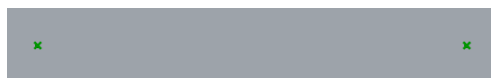
Figure 85: In the modelspace, the user only needs to reference two points into the Grasshopper script. These are the endpoints of the unstressed SMA, one fixed and one to attach the bias object. The other inputs are all numerical.
