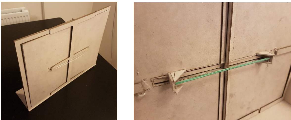
Figure 102: a) 1:10 prototype, showing the exterior side of the façade module. The green elastic band represents the SMA element b) the hardware on the other side, with an elastic band representing the bias force that always applies tension into the SMA wire
