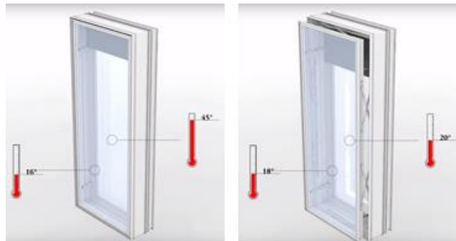
Figure 36: When the temperature in the cavity exceeds 23°C, the paraffin wax actuators push the outer pane out by 5cm. The window self-closes when temperature cools back down. 9
