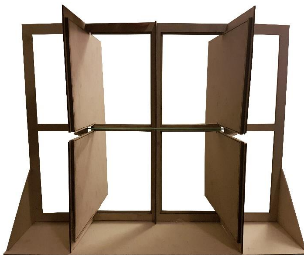
Figure 103: testing of the opening motion with the 1:10 prototype
