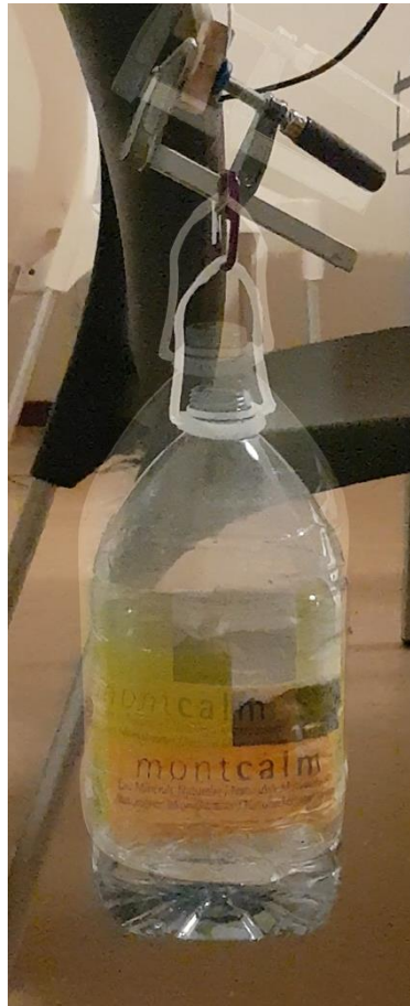
Figure 113: Two overlaid snapshots from a voltage testing video. The 4kg mass being used to stress the nitinol wire to 200MPa. When an 18V current is passed through the wire, it shortens and raises the mass as shown
