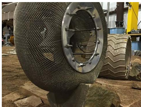
Figure 55: A wheel made of SMA, designed to be used in the austenite phase to traverse a range of alien terrains (NASA)
