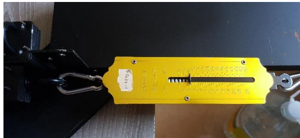
Figure 115: A closeup of a spring-scale device. K-value = 4298 N/m
