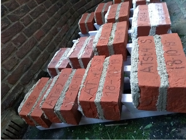
Fig. 3. Brick-mortar specimens in outdoor conditions.
