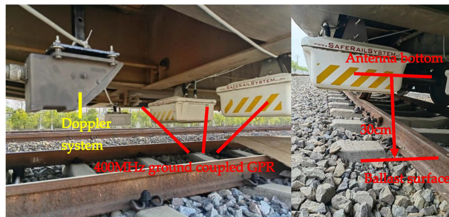
Figure 2. The subgrade status inspection vehicle with a three-channel GPR antenna group.
