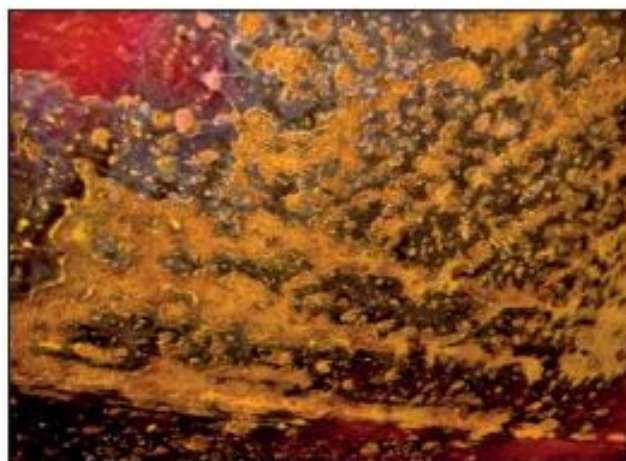
Figure 1.3: Coating deterioration after 4 years of service with conventional hull coating like a foul releasing coating or anti fouling coating [93]
