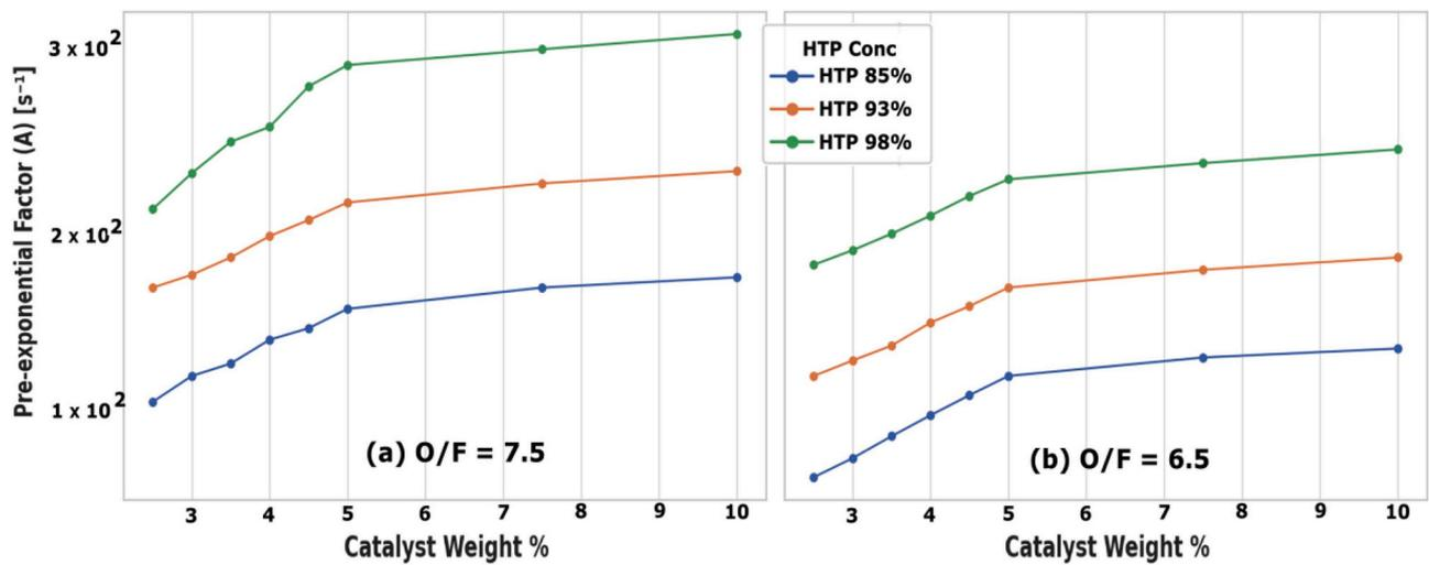
Fig. 9. Apparent pre-exponential factor (A) as a function of catalyst loading and HTP concentration for (a) O/F 7.5 and (b) O/F 6.5, demonstrating the kinetic effects on hypergolic ignition and illustrating the diminishing returns beyond 5 % catalyst weight.
