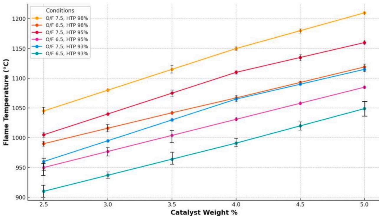
Fig. 10. Variation in post-ignition flame temperatures as a function of catalyst weight percentage for different O/F ratios and HTP concentrations. Error bars represent the standard deviation ( $n = 5$ ); where not visible, error bars fall within the area of the data point.
