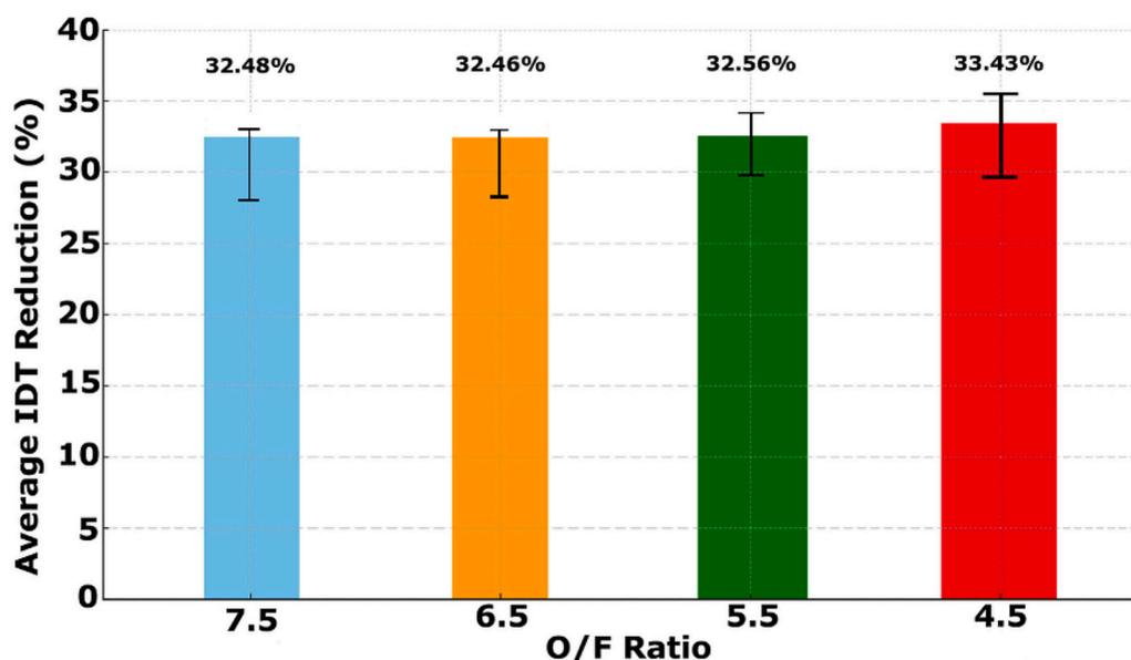
Fig. 4. Average percentage reduction in ignition delay time when initial fuel mixture temperature is increased from 20 °C to 50 °C, categorized by O/F ratio. Data represents only paired conditions where ignition was successful at both temperatures ( $N \approx 20$ –40 unique conditions per bar). Error bars represent the standard deviation.
