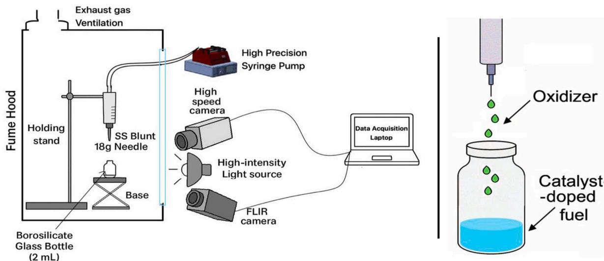
**Fig. 1.** Schematic illustration of the open-air drop test apparatus and the propellant dispensing method. The setup (left) includes a precision syringe pump with an 18 G needle for oxidizer dispensing into a 2 mL borosilicate glass bottle, all housed within a fume hood, with high-speed and FLIR cameras for data acquisition. The right panel depicts the oxidizer droplets impacting the catalyst-doped fuel pool.
