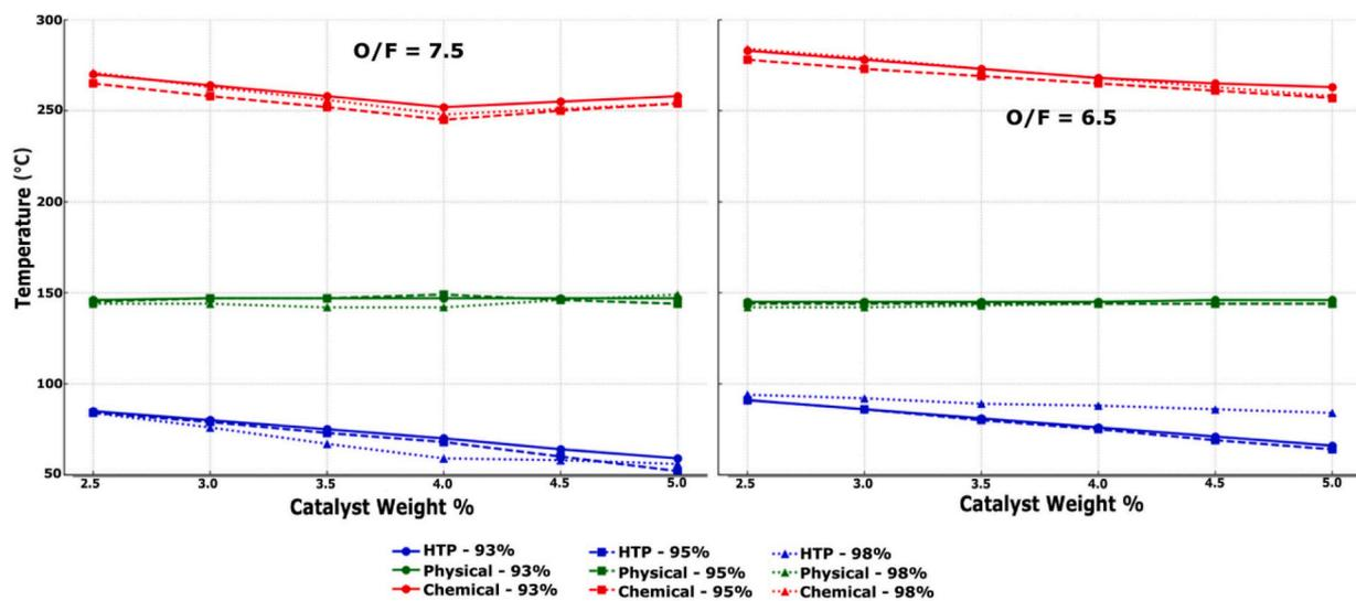
**Fig. 8.** Characteristic temperatures during HTP decomposition, physical mixing, and chemical reaction phases as a function of catalyst loading, HTP concentration, and O/F ratio. The maximum observed standard deviation was  $\pm 8$  °C; consequently, error bars are frequently smaller than the data markers. Note: A systematic uncertainty of  $\pm 20$  °C applies to absolute temperature values due to emissivity variations.
