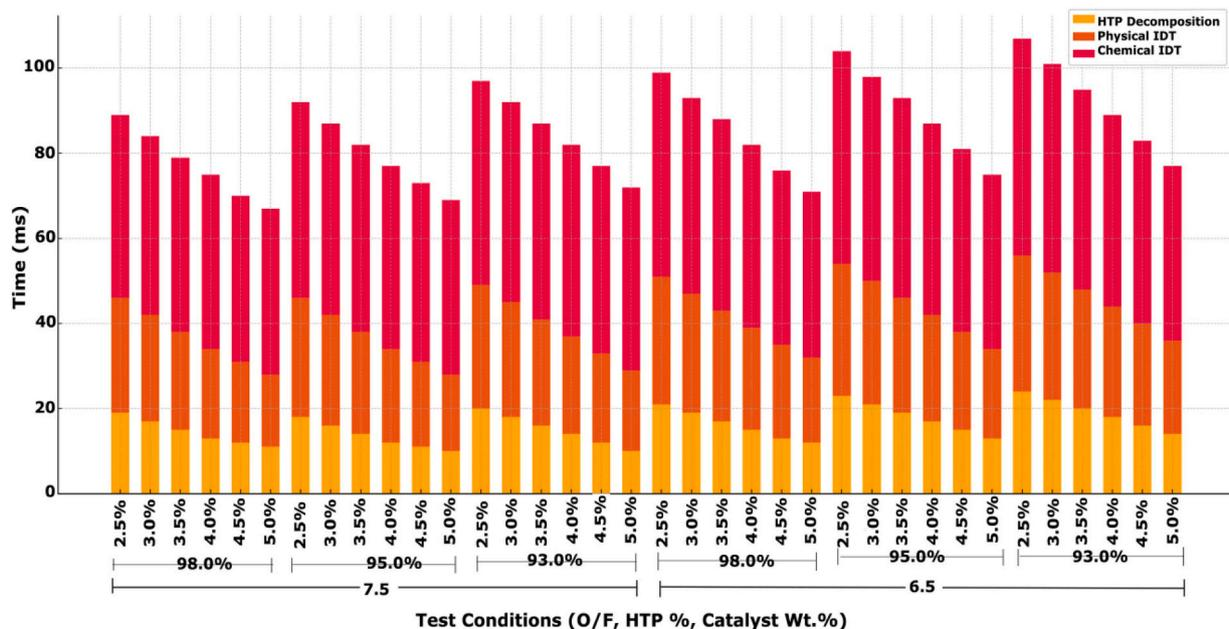
**Fig. 6.** Contributions of HTP decomposition, physical, and chemical phases to total ignition delay time (ms) across varying HTP concentrations and catalyst loadings for O/F 7.5 and O/F 6.5.
