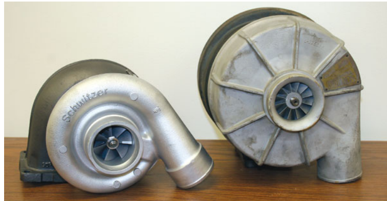
Figure 1.2: The current Schwitzer-BorgWarner model S3 on the left has a slightly higher airflow range than the older Schwitzer model made in the 60's for Cummins Engine Company. While the intended applications are different, it's easy to see the dramatic design differences that have come about from computer-aided designs, improved materials and manufacturing processes (source: Diesel Injection Service Company, Inc.)
