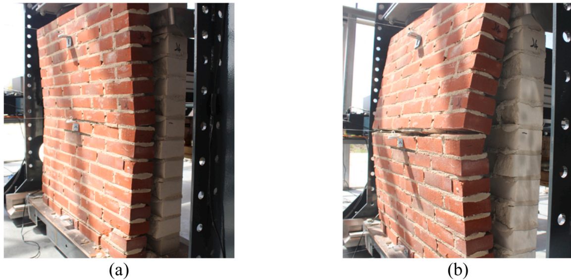
Fig. 9. Rocking behaviour of TJ4 under pulling (a) and pushing (b).
