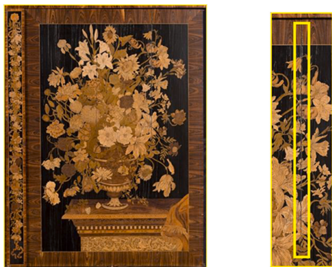
Fig. 1. The development of a vertical crack along the adhesive joint of the panels in a decorated cabinet door. Jan van Mekerén, The Netherlands, c. 1700. Oak door: 110 × 80 × 3.5 cm, located in Castle Amerongen (The Netherlands), courtesy of René Gerritsen.
