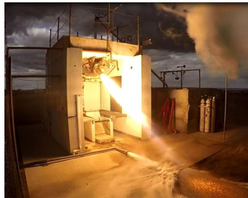
Figure 2.6: Rutherford engine test at Rocket Lab's test facility - Mass flow approximately 7 kg/s (see Footnote 6, 7)
