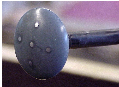
figure 3-6 Close up of the probe of the EMS.
