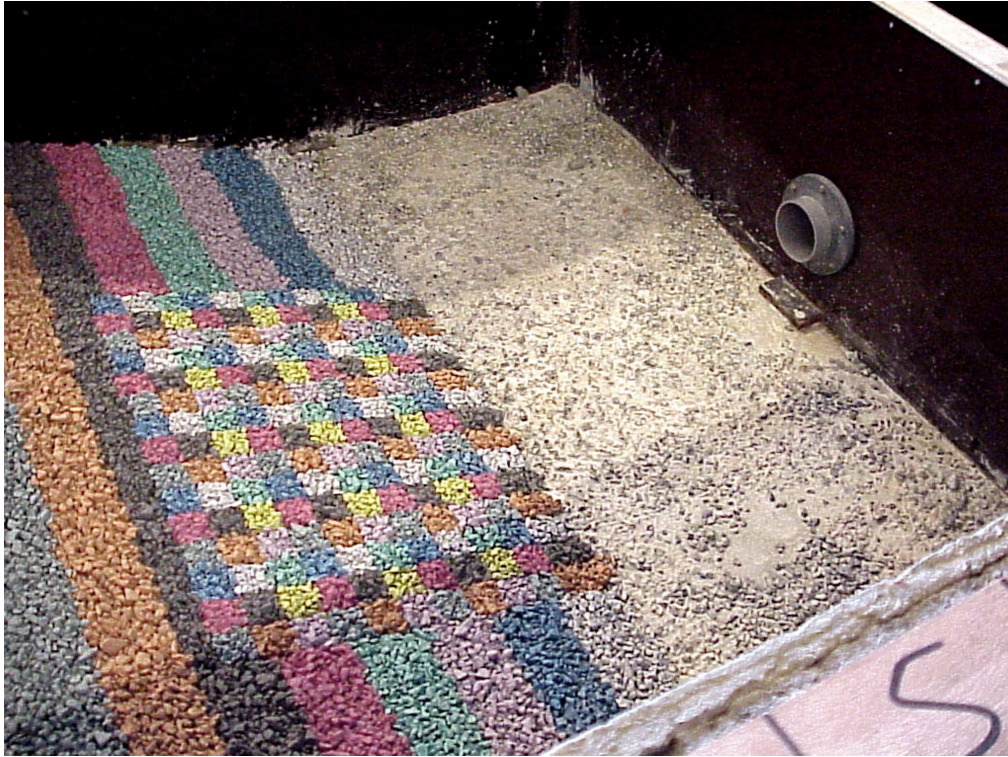
figure B-1 The ducted propeller and the coloured stones on the slope.
