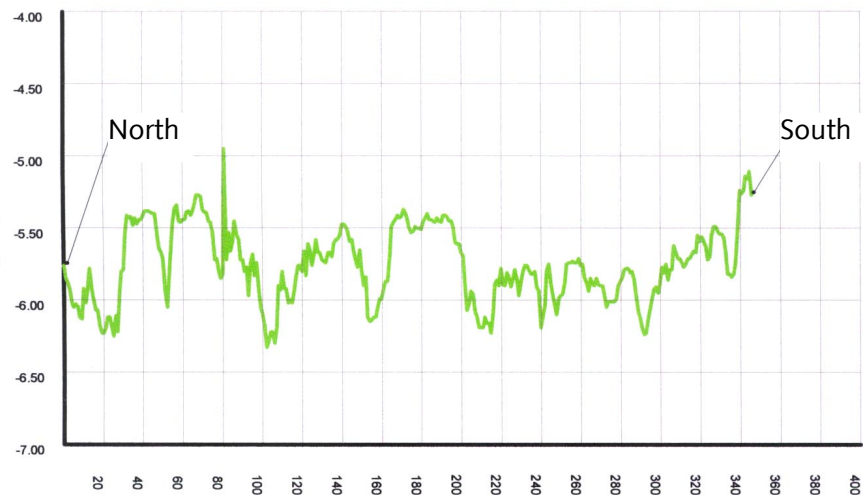
figure 6-4 Bathymetry at Maarsse. All values are in metres. Reference level for depth profile (5 [m] outside the quay) is NAP.
