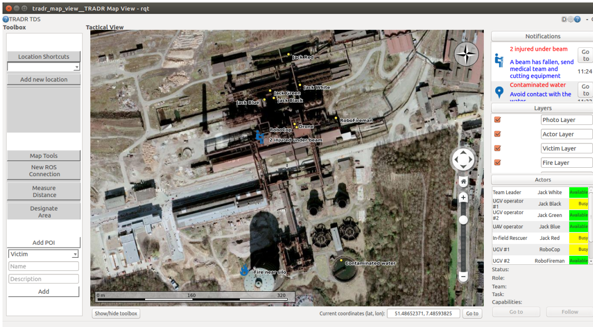
Figure 5.6: Interface of the TDS with multiple points of interest on the map, including actors. This interface is sized to a bigger screen size, such as a desktop or laptop with all information views open
