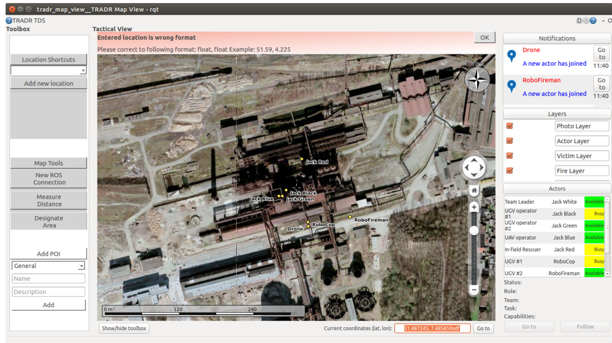
Figure 5.7: Interface of the TDS with a non-invasive error message showing, caused by an incorrect input
