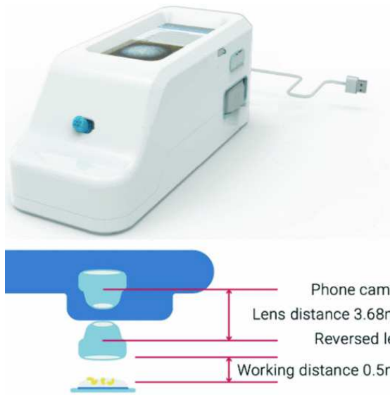
Figure 3.4: Schistoscope SP (up) with working principle of sensor and lens combination (down).
