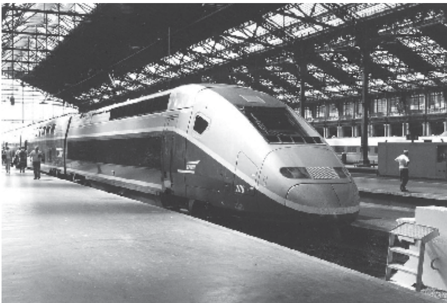
Figure 1.1 Double-decker TGV Duplex high-speed train at the Gare de Lyon, Paris
