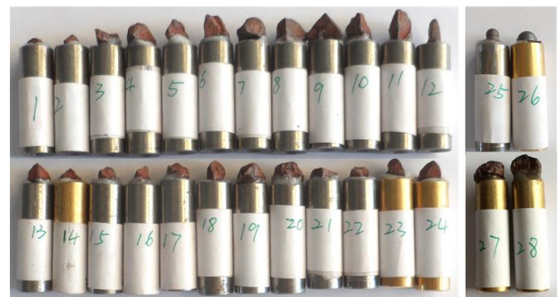
Fig. 6. Particle pins used for pin-on-disk wear test.
