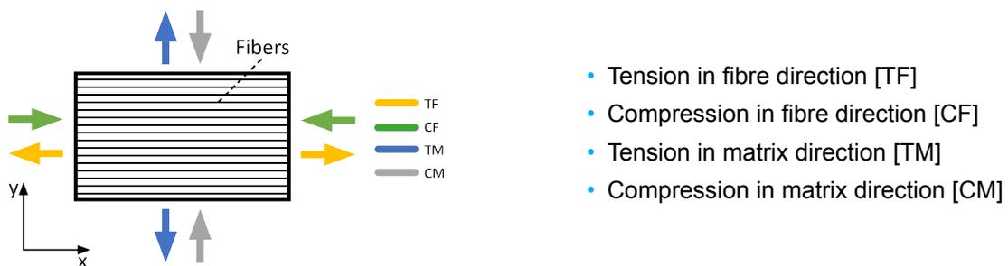
Figure 3.4: Schematization of the four different loading directions
