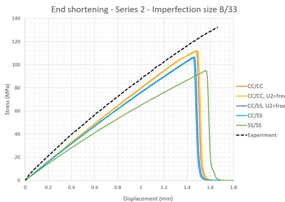
Figure 6.21: Stress-end shortening curves for series 2 with imperfection size B/33
