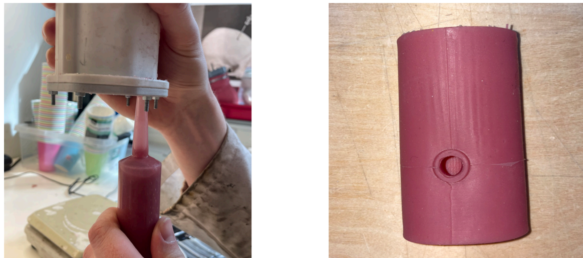
Figure 26: Left: fill mould with large amount of air. Right: produced silicone part
