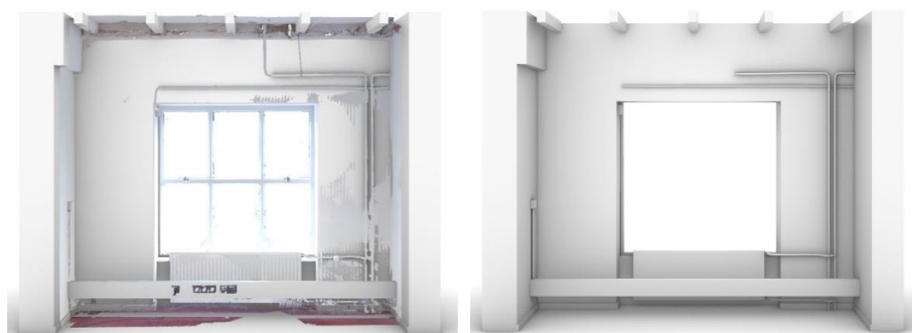
Figure 48 The building elements modelled over the point cloud in Rhinoceros
