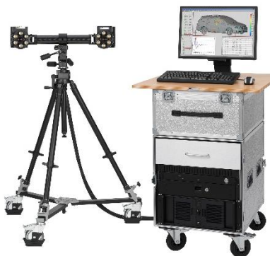
Figure 22 GOM Pontos Live, a mobile optical 3D measuring system consisting of two high-speed camera. Retrieved from www.r-design.hu/hu/pontos-rendszer
