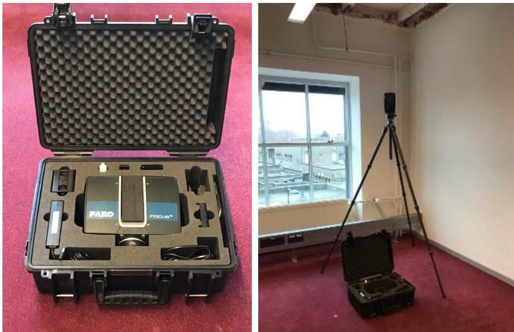
Figure 42 The scanning equipment is easily portable with the items fitting a briefcase along with a lightweight carbon fibre tripod stand
