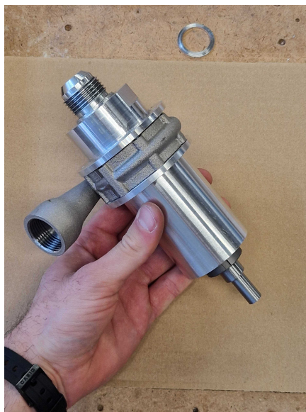
Figure 2.12: Assembled DARE fuel pump. Image courtesy of DARE.
