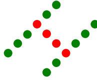
Figure 3.11 Example of a spurious pattern with the slanted line, forming a slanted “H” due to the combination of desired states (in green) and static states (depicted in red), which can form a bridge between two lines.
