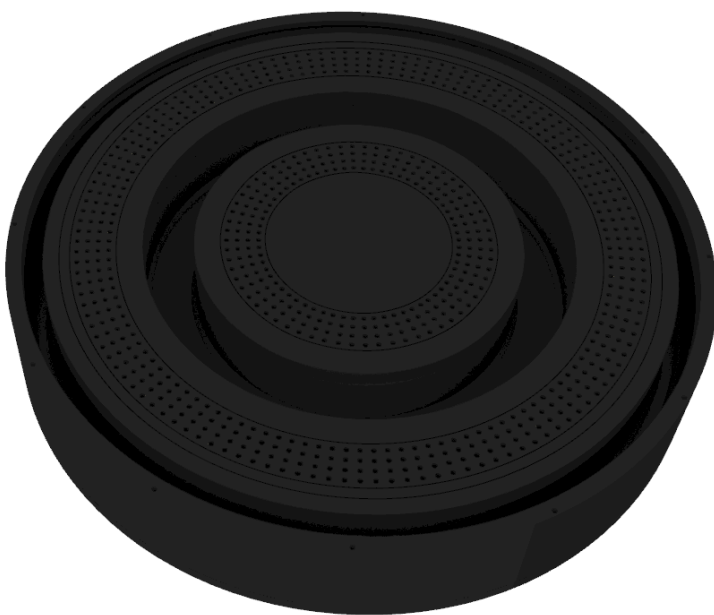
Figure 22 The POM-block with silica grains for the MLA (without air hoses).
