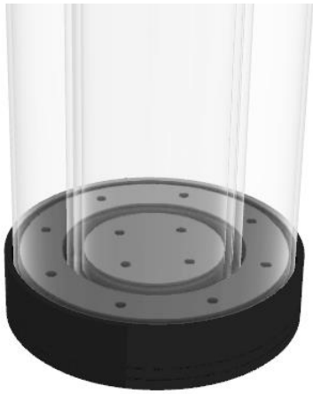
Figure 3 The glass will be placed in a POM-block.
