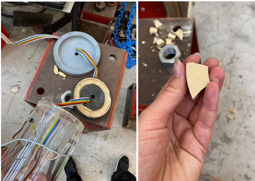
Figure 57 The second time to try-out the way of injecting Hilti. It was possible to pull out the glass later on (left). In this figure the Hilti was pushed out of the POM and a part of the bottom is shown which was well-distributed in the POM-block (right).
