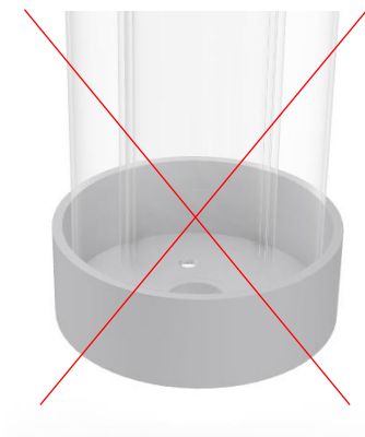
Figure 2 No direction connection between glass and steel
