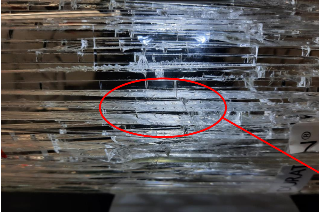
Figure 52 Straight cracks at the outer tube, and a few perpendicular cracks appeared when the force was taken off - sample 6.
