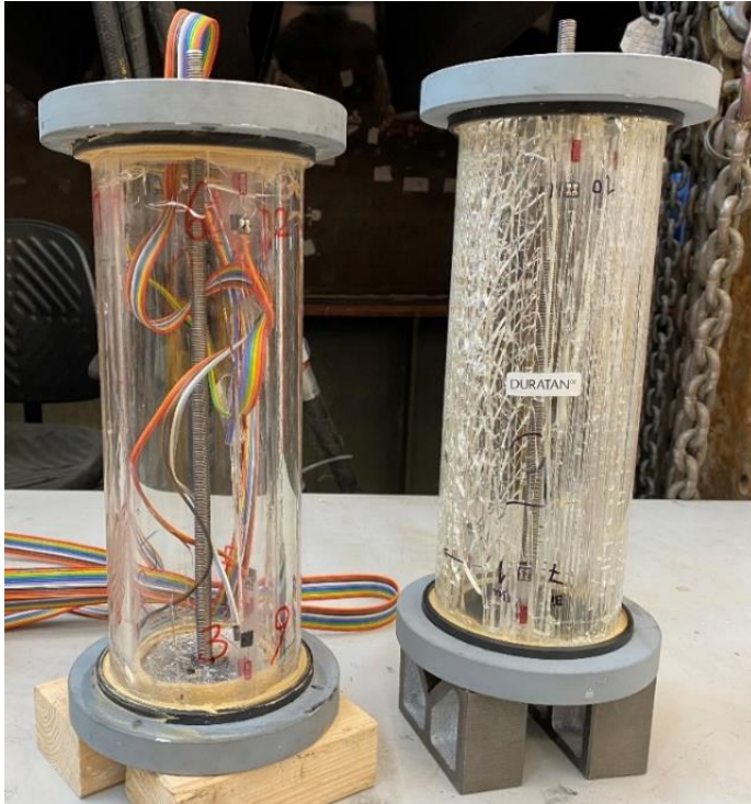
Figure 81 Left a cracked annealed glass sample (sample 2) and right a heat-strengthened glass sample (sample 5).
