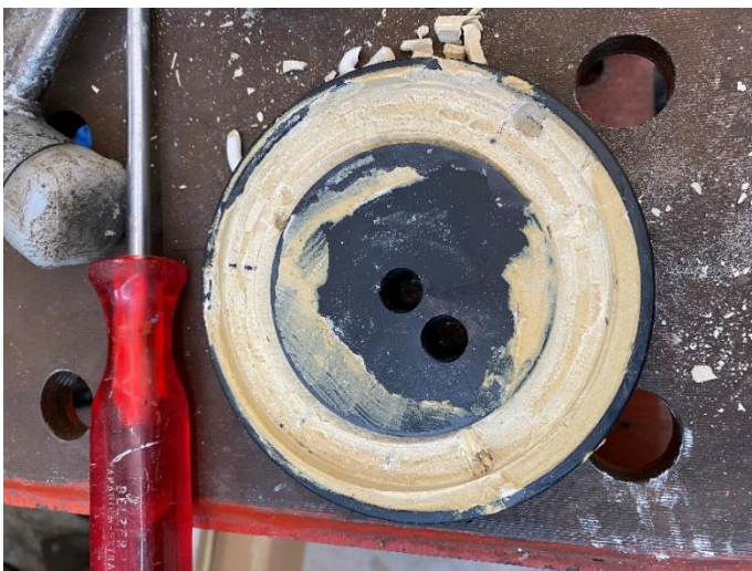
Figure 3 The connection parts and the Hilti remained intact.
