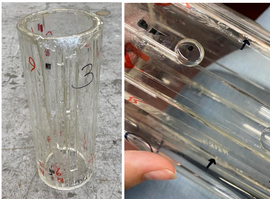
Figure 25 The first few cracks are visible of the cracked sample (left). A few stopped cracks are visible: black arrows (right).
