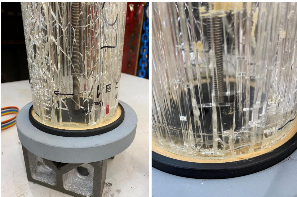
Figure 55 The Hilti mortar was properly injected – sample 5.
