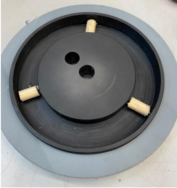
Figure 15 The timber pieces glued into the POM-block.
