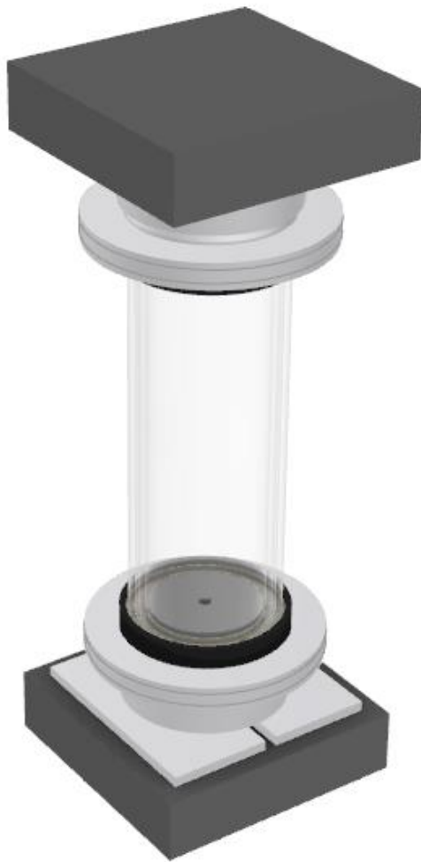
Figure 12 3D view of the sample with a length of 300 mm for the test setup.
