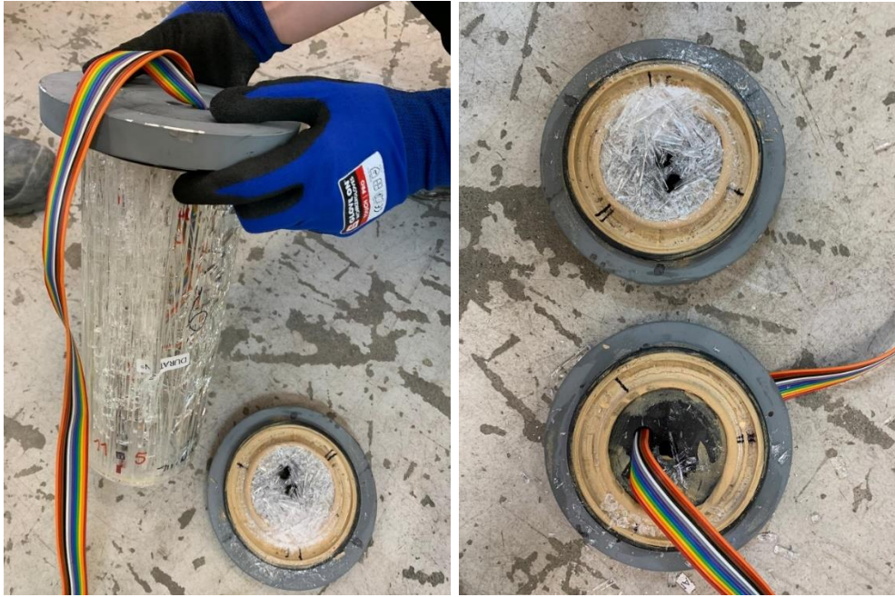
Figure 32 The glass sample taken out of the connection after testing.
