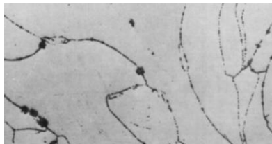
Figure 21 Crystallization when the temperature is too low (Roeder, E. 1971).
