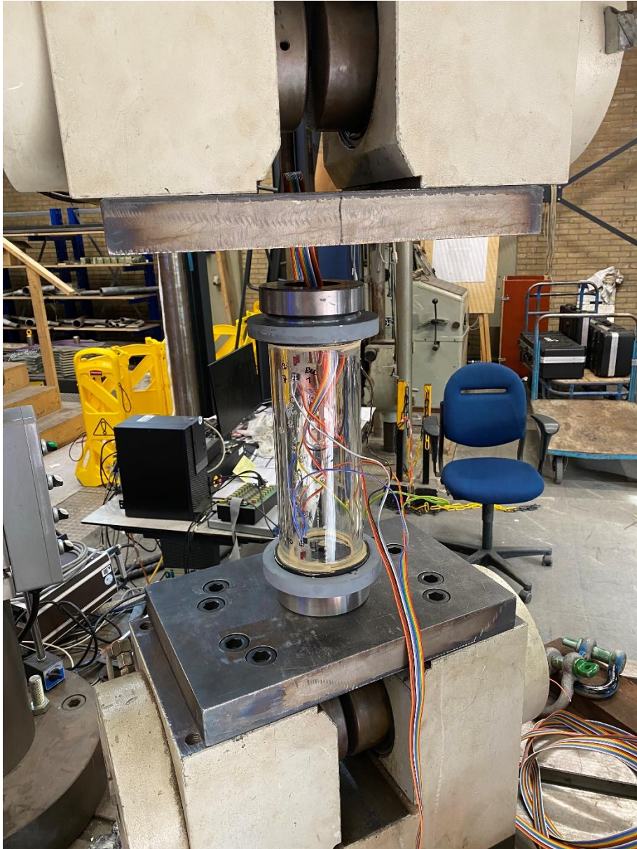
Figure 22 The wires from the inside sensors can go through a hole in the top plate to the computer.
