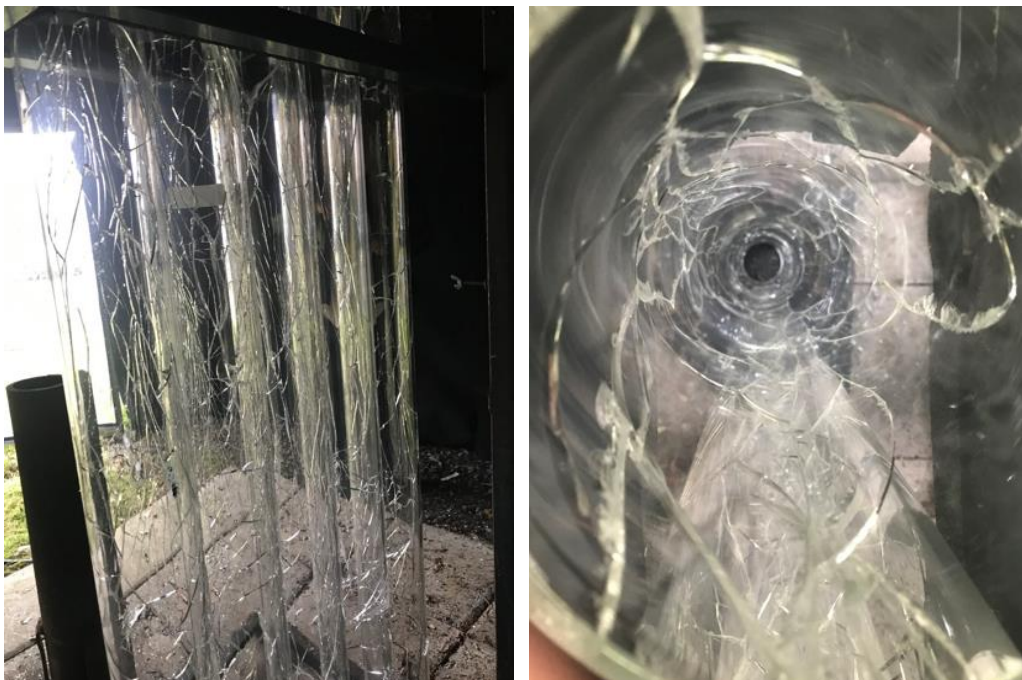
Figure 50 Blast test on DURAN® tubes (left the outside view, right the inside view) (SCHOTT internal. 2019).
