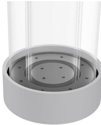
Figure 4 The POM-block will be placed in the steel shoe.
