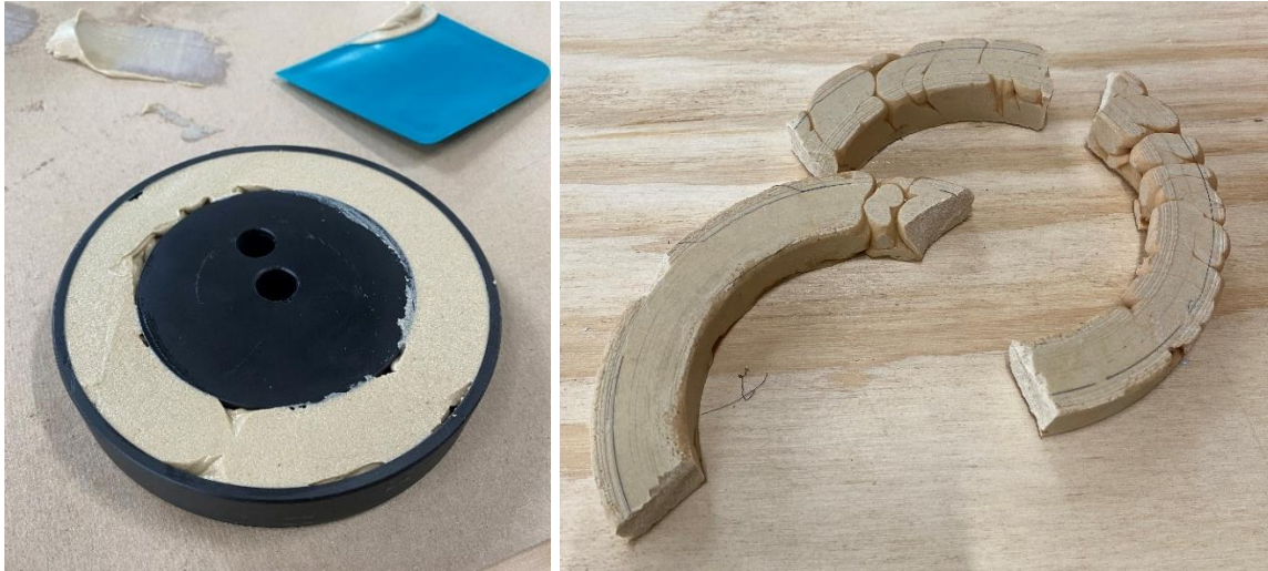
Figure 56 The first try of injecting Hilti in a POM-block (left). The Hilti was taken out of the POM and is shown at the bottom side (right).
