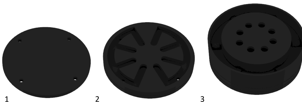
Figure 12 POM-block to regulate water with three layers
