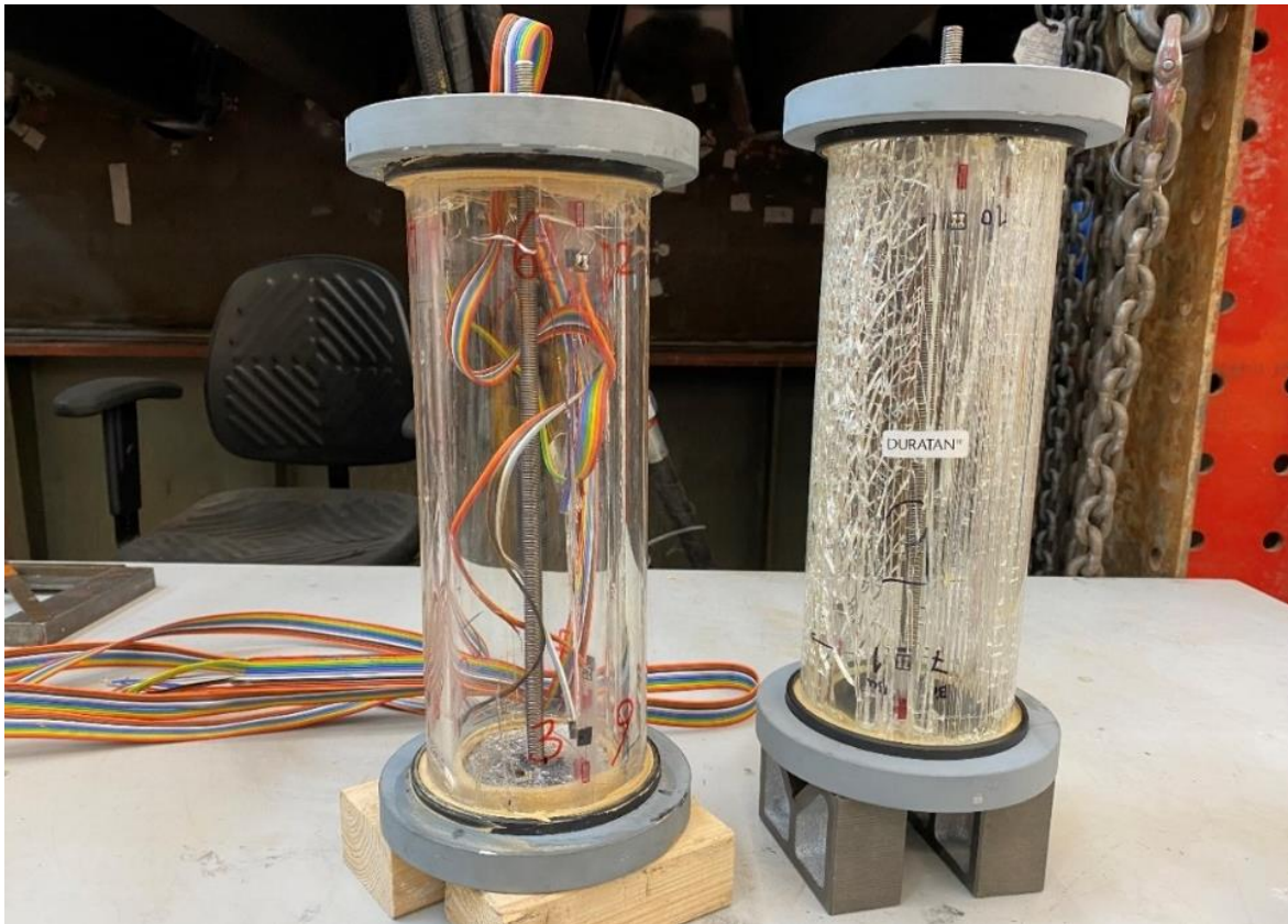
Figure 62 The cracked result from an annealed sample – sample 2 (left), and from a heat-strengthened sample – sample 5 (right).
