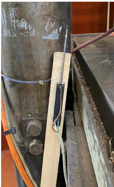
Figure 8 Sensor to control the displacement in z-direction during testing.
