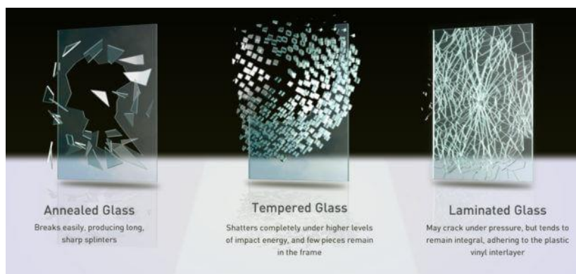
Figure 28 Breaking patterns of annealed, tempered, and laminated glass panes (Crystalia Glass Architectural glass & metal. 2020).
