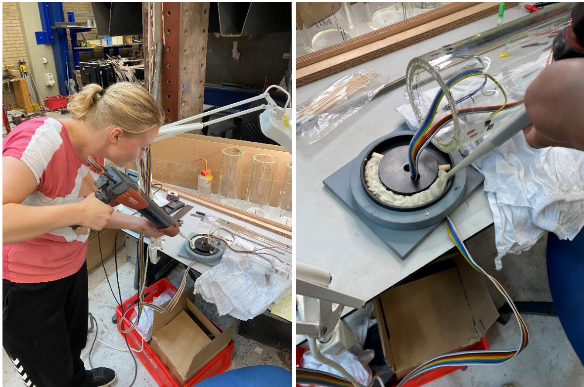
Figure 17 Injecting the Hilti mortar for one of the samples.
