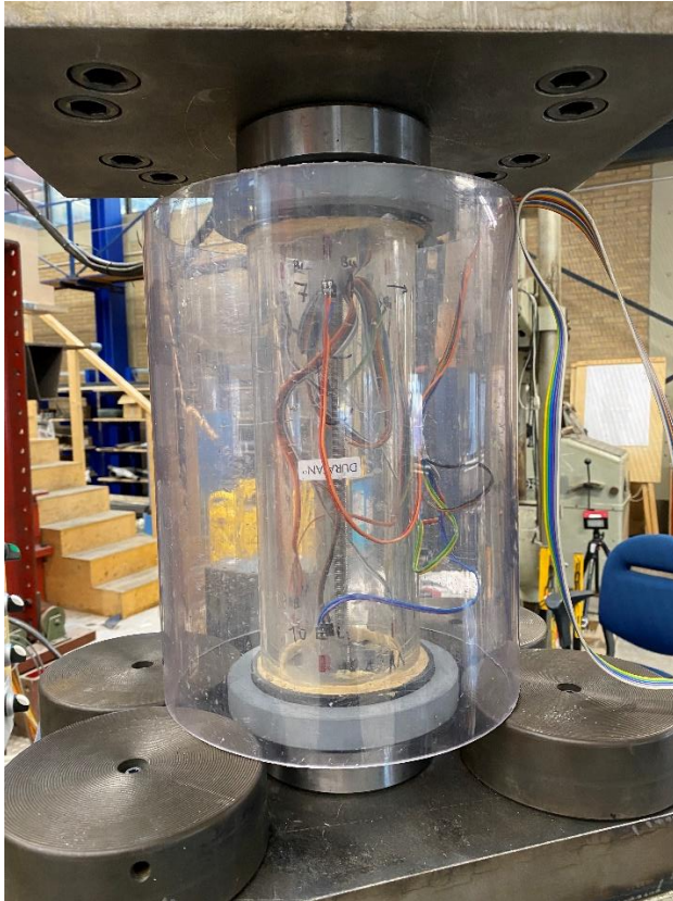
Figure 2 In the first test, a plexiglass enclosure was used to ensure safety (later on plexiglass panels were used to stand behind. In this way the sample itself was more visible during testing).
