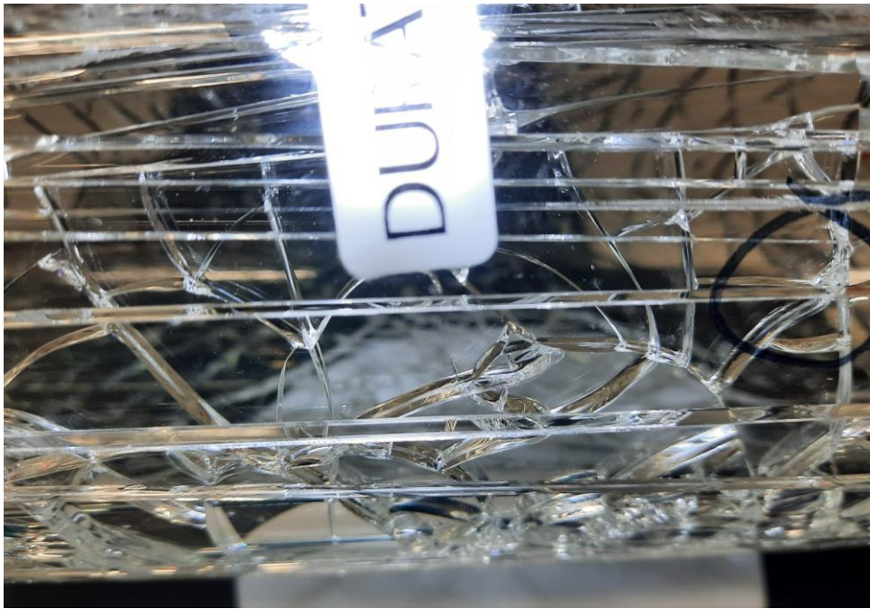
Figure 48 At the outer tube straight cracks are visible and the inner tube cracked into smaller pieces – sample 6.
