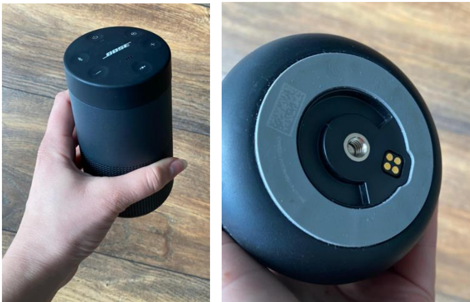
Figure 14 Bose-sound speaker with a threaded connection into plastic.
