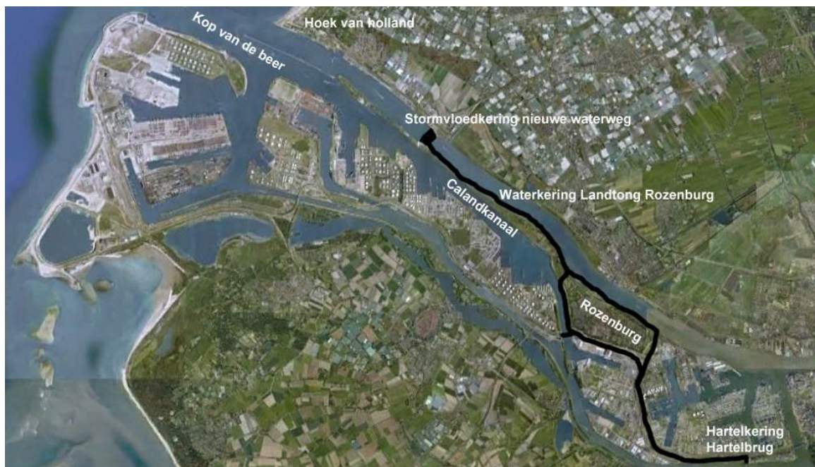
Figure 20: the Europoort barrier (Rijkswaterstaat, 2012). Dike segment part of the Europoort barrier highlighted in black.
