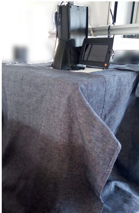
Figure 3.4: Protective covering from glass wool and thick cloth built around the IR camera to reduce capturing of stray signals.
