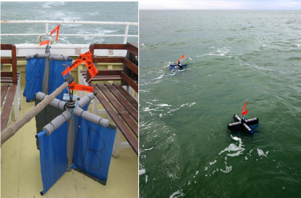
Photograph 10.2 GPS-Drifters constructed and used for measurements
